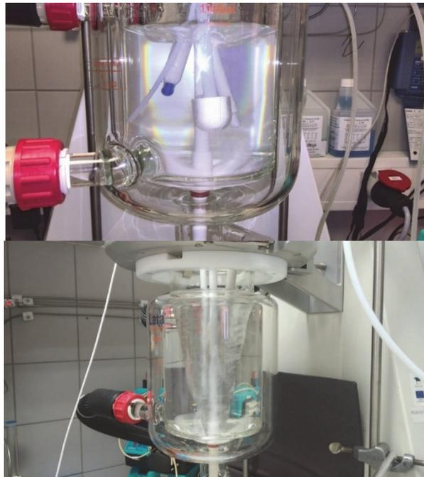
Figure 5. *Mixing at 250 rpm (up) and at 650 rpm (down).*
