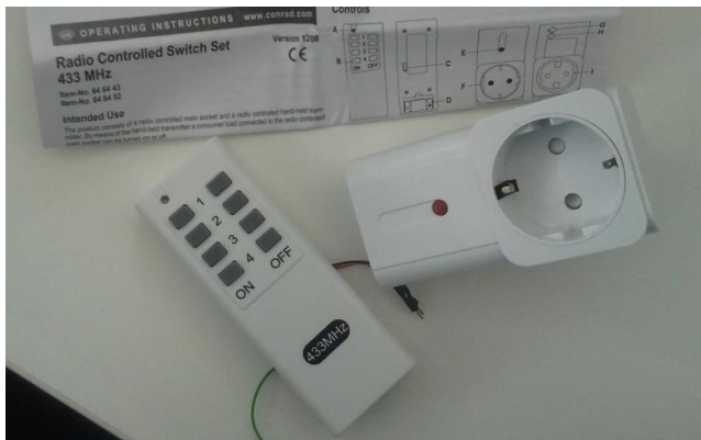
Figure 12. Radio controlled switch set
