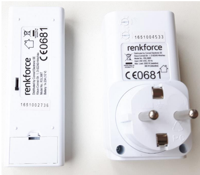
Figure 18. Radio controlled power socket
