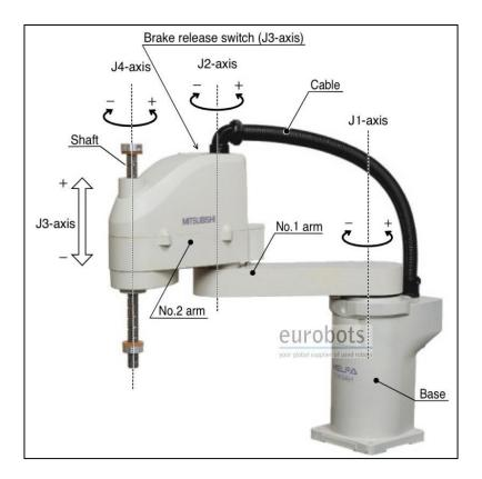
Figure 5. Photo of SCARA robot with markings
