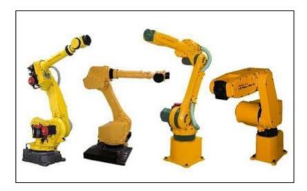
**Figure 7.** Real pictures of 6-axis robots
