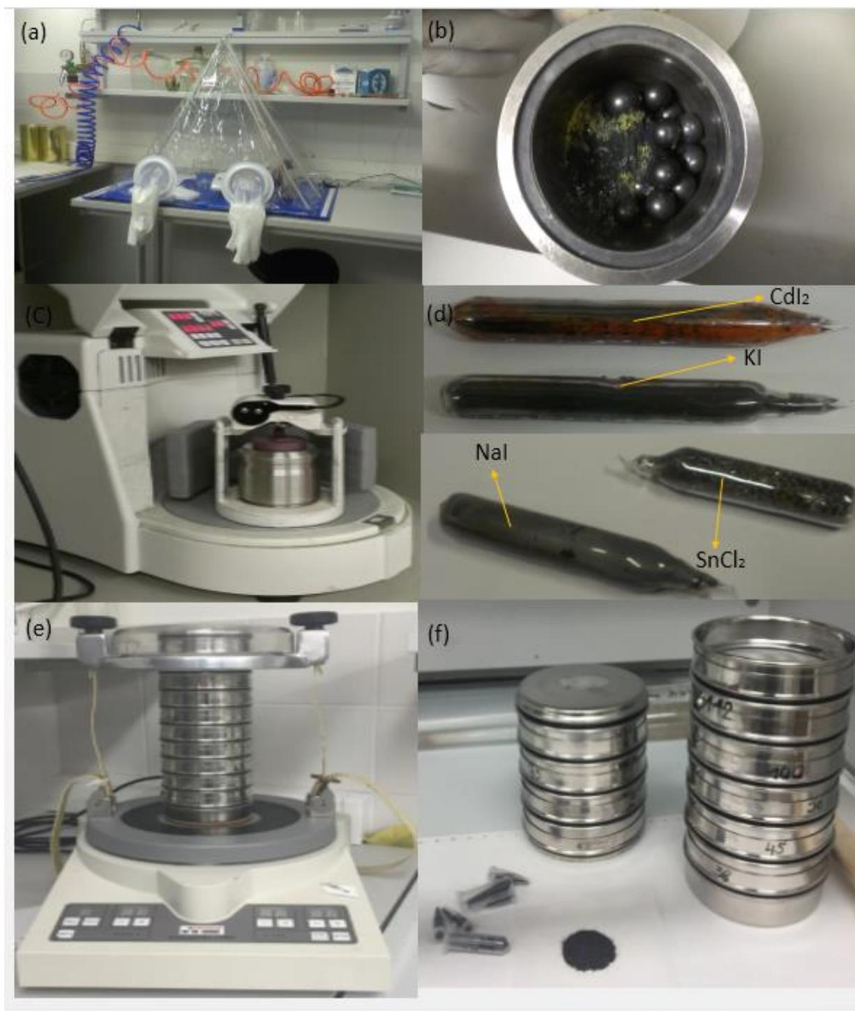
Figure 3.1 Experimental steps of the monograin powder preparation process: (a) glove box saturated with Nitrogen gas, (b) the precursors were milled mechanically to ensure homogeneous mixture, (c) the ball milling system, (d) annealed samples with different flux materials showing their different colors and appearances, (e) the sieving machine containing different size of sieves (ranging from 38 $\mu$ m-125  $\mu$ m), (f) monograin fractions obtained from different sieves after sieving.
