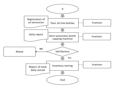
Figure 4 Diagram of oil flower manufacturing process in NAZGOL company II
