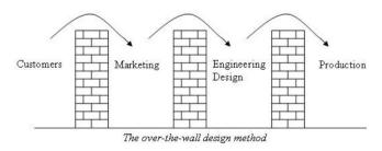
Figure 7 the over-the-wall design [26]
