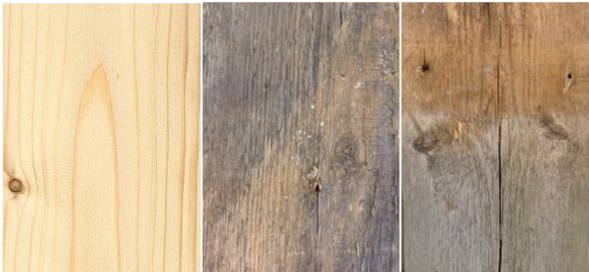
Figure 28. European spruce surface colour and appearance as a fresh solid wood and as a reclaimed wood. Left one is fresh spruce wood (Wood-Database) and images from reclaimed wood test specimens are in the center and on the right.
