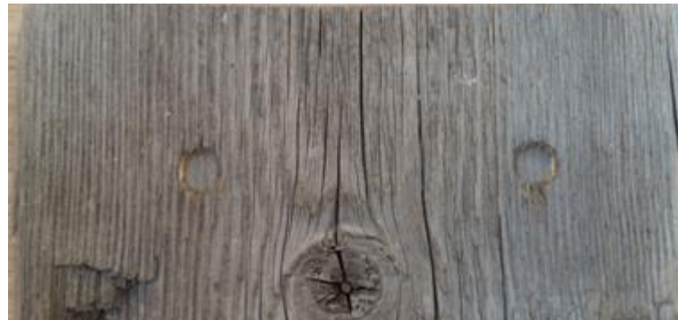
Figure 44. Spruce wood surface after testing Janka hardness.
