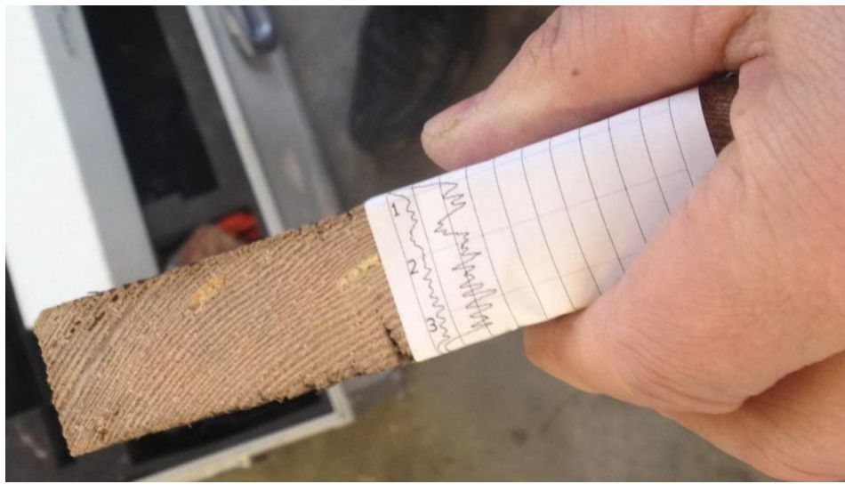
Figure 27. RESISTOGRAPH® identifies all of the annual rings and wood damages .
