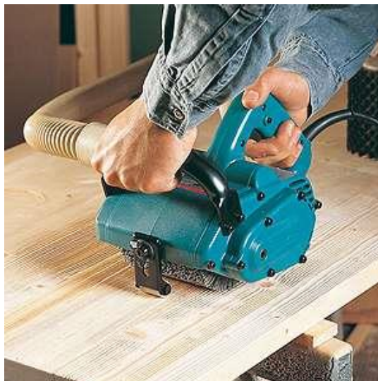
Figure 13. Brush sanding machine (Woodworking machinery).
