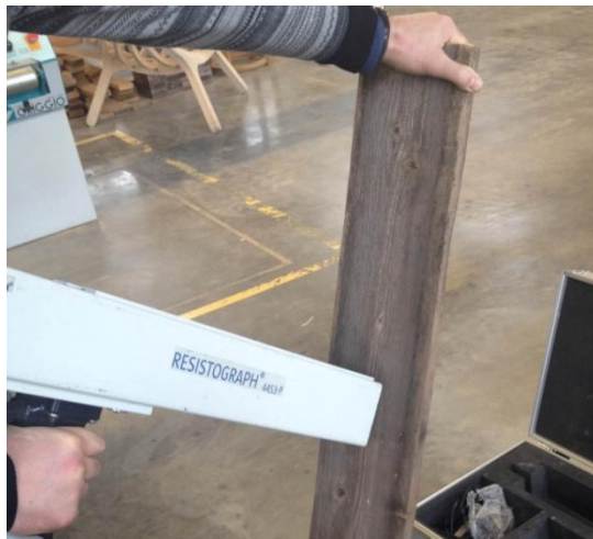
Figure 26. Measuring with RESISTOGRAPH®.
