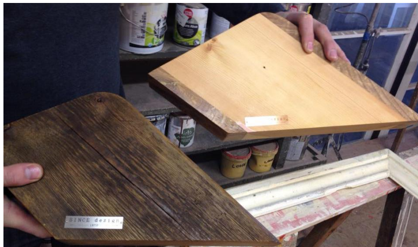
Figure 17. On the left is a regular reclaimed wood surface, on the right reclaimed wood processed with a planer (samples from SINCE Design OÜ).
