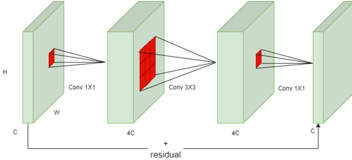
Figure 15: Operation method for Inverse residual block.
