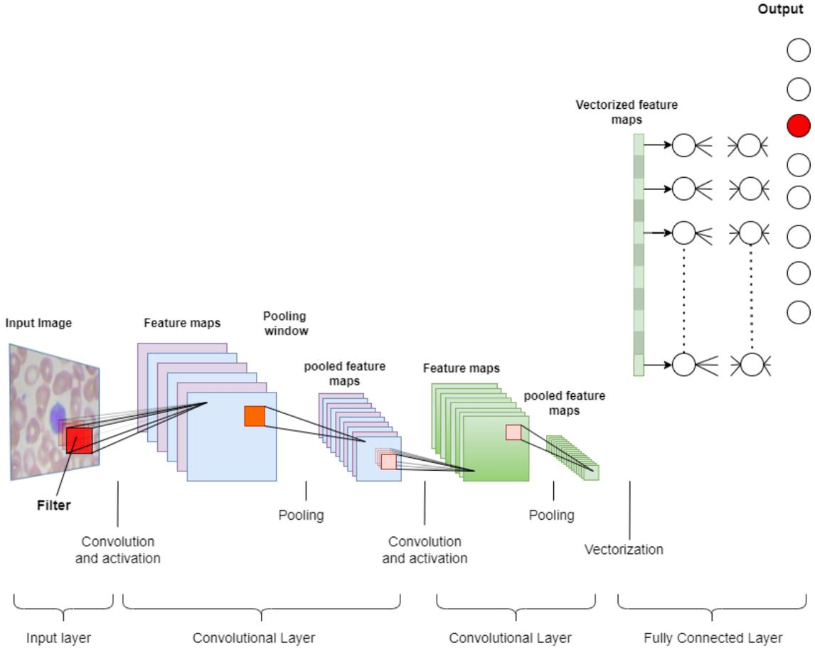
Figure 8: Building blocks of a typical CNN. A slight modification of a figure in [60], courtesy of the author.
