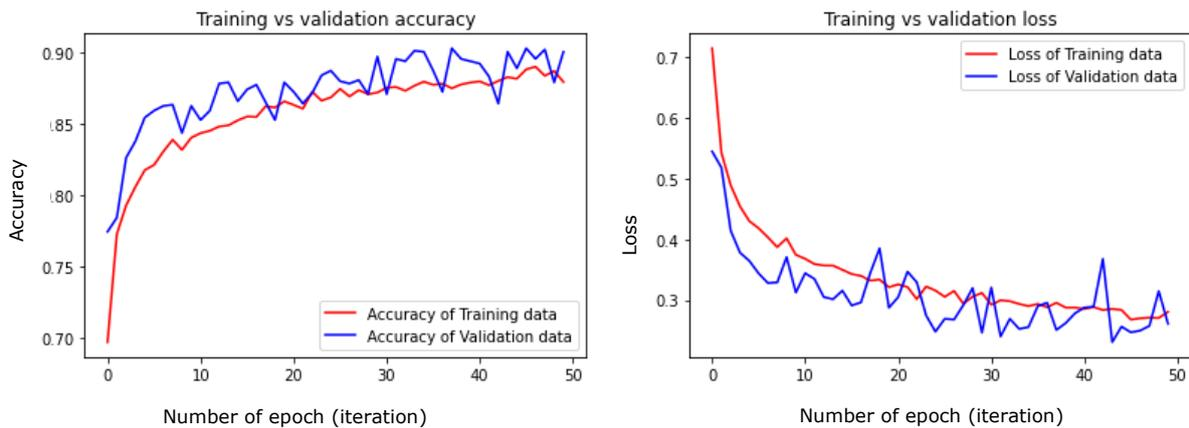
Figure 36: Learning curve of Model 2. The X axes represent the epochs (“training iterations”) and the Y axes represent the accuracy (max value is 10) and loss.
