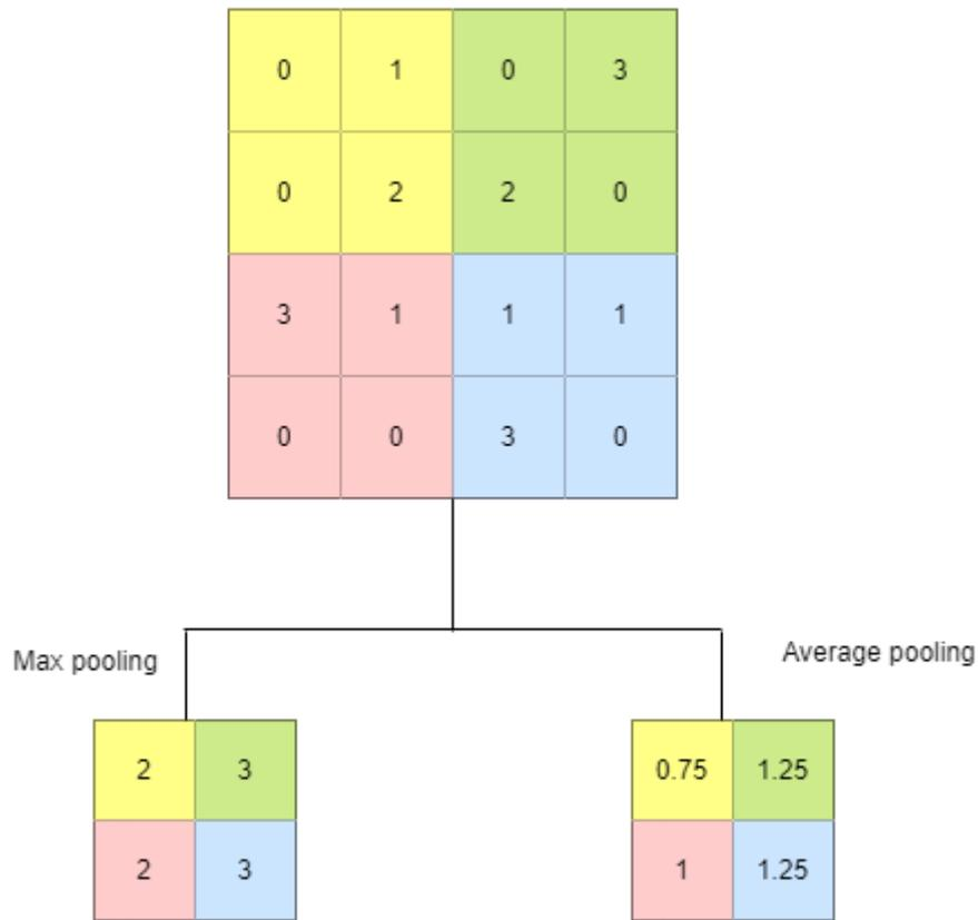
Figure 9: Process of Max pooling and Average pooling.
