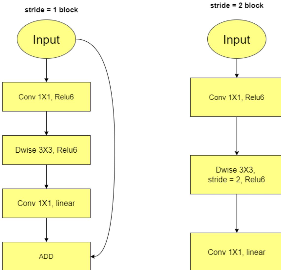
Figure 16: Convolution algorithm of MobileNetV2 [72]
