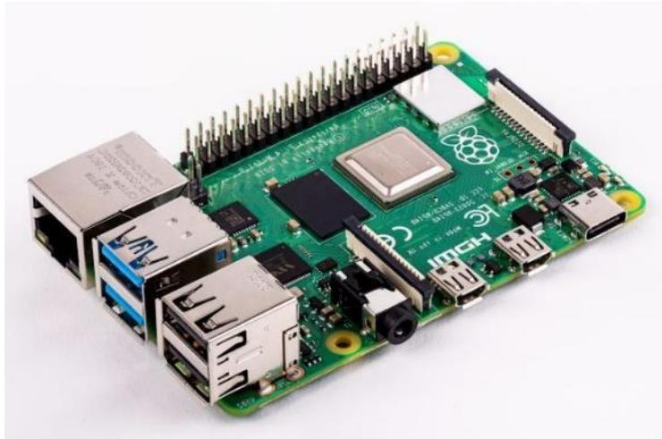
Figure 19: Photograph of the Raspberry Pi 4 (Model B) used in this MSc thesis.
