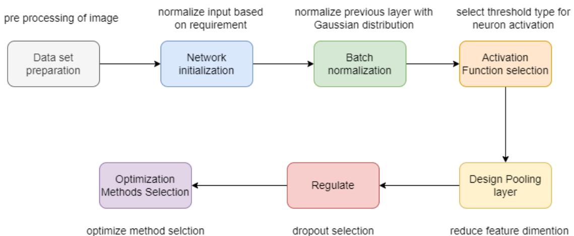
Figure 22: Flow diagram for CNN model development used in this MSc thesis
