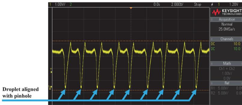
**FIGURE 19.** Oscilloscope screen capture of recorded amplified, inverted photodiode voltage during droplet generation with chip variant C, at a rate of  $\sim 500$  Hz. Droplet alignment with the pinhole noted with blue arrows (at the “troughs”). Instability in the droplet production rate is recognizable by the varying time gaps between the „troughs“.
