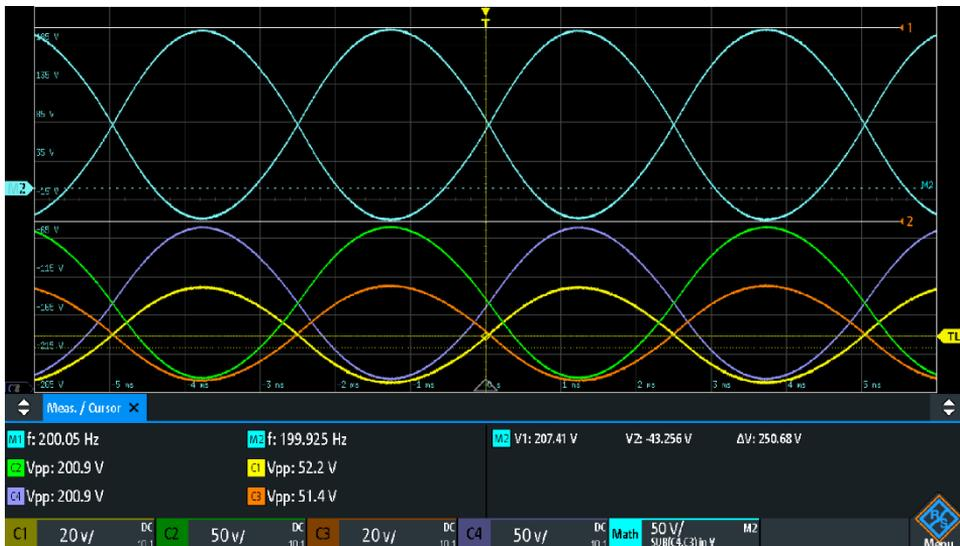
Figure 37. Custom PPD unloaded output waveforms at  $\sim 200$  Hz and  $\sim 250$  V<sub>pp</sub>.
