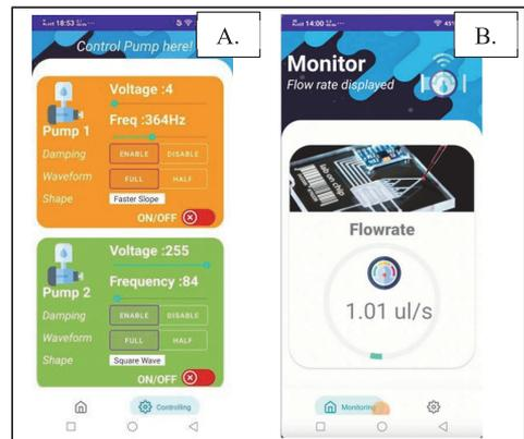
Fig. 4. GUI: Smartphone application showing instrument control page where the user can configure parameters (A.) and sensor monitoring page (B.)
