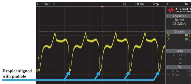
**FIGURE 21.** Oscilloscope screen capture of recorded amplified, inverted photodiode voltage during droplet generation at a rate of  $\sim 200$  Hz. Droplet alignment with the pinhole noted with blue arrows (at the “troughs”).
