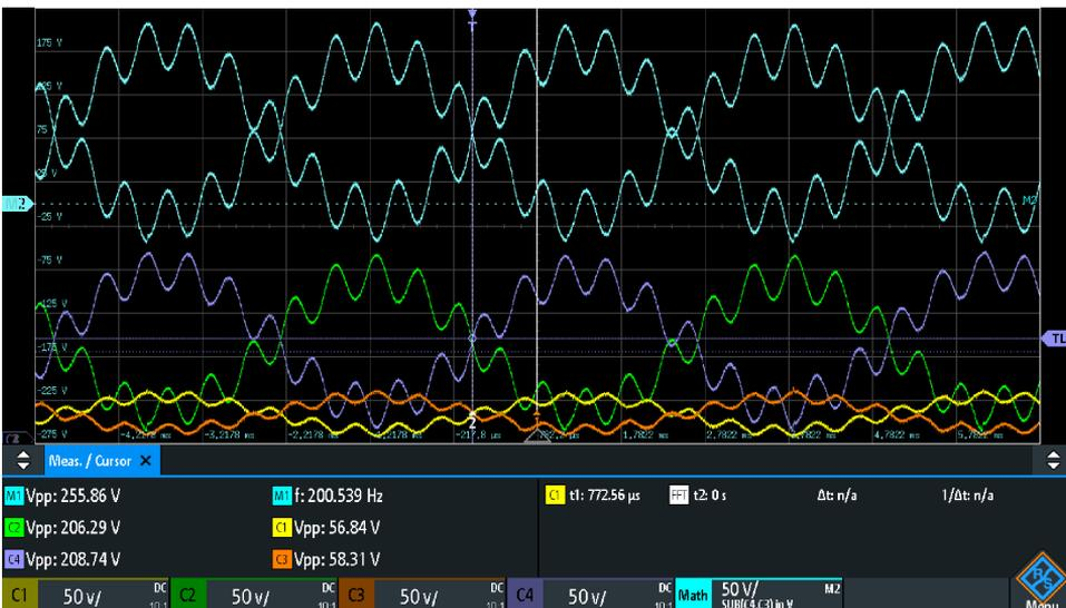
Figure 39. WF1 (~200 Hz) and WF2 (~2000 Hz) summed result.
