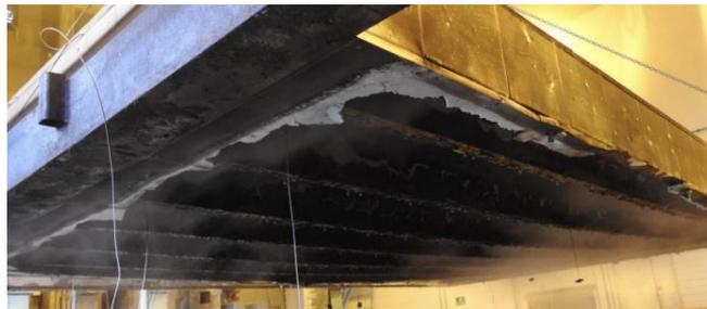
Figure 5.1-3 Exposed side of the test specimen after it was extinguished with water and cooled down [8]
