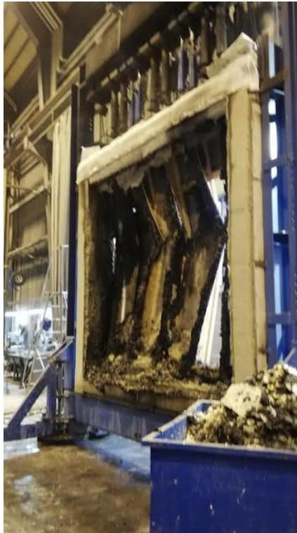
Figure 5.2-4 Buckling out of walls plane after the fire exposure
