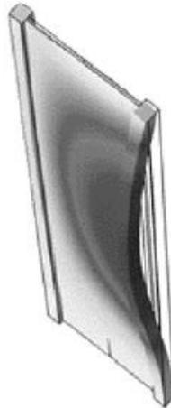
Figure 4.3.4-1 Buckling in walls plane for Case 3 [1]
