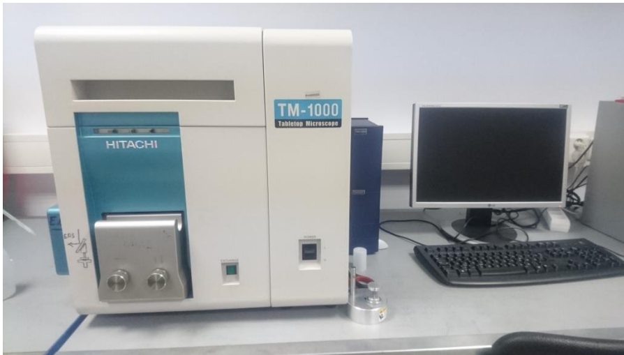
Figure 14. Hitachi TM 1000 SEM Tabletop microscope
