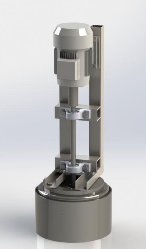
Figure 11. 3D model of improved hydro-abrasive (slurry) tester
