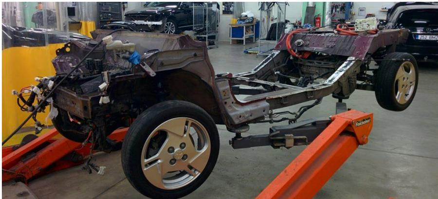
Figure 3.7 ISEAUTO components under the body shell [25]
