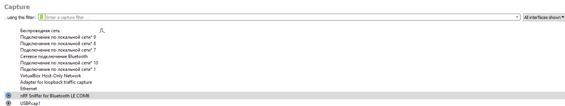
Figure 7: Wireshark interface after successful setup of the BLE tool
