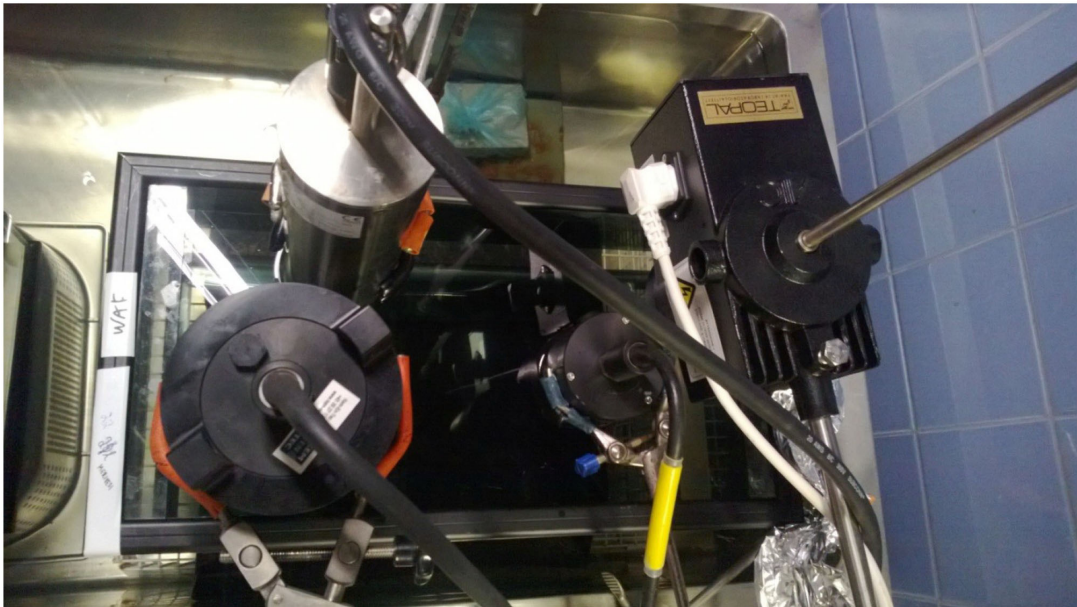
FIGURE 1 | Above view of the experimental set up. Instruments: TriOS EnviroFlu-HC (with metallic cover, upper part), Turner C3 (with black cover, left) and UviLux (black cover, right). The electric motor of the stirrer is at far right. Photograph: Harri Kankaanpää.
