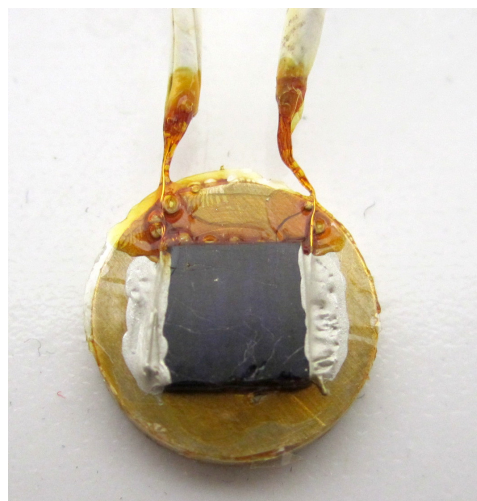
Figure 13: \text{LiCoPO}_4 sample with gold wires attached for a high voltage experiment. The sample is electrically isolated from the \varnothing 10 mm sample disk by a Mylar film. Gold wires are glued to the sides of the sample with a silver conductive paste and additionally glued with a non-conductive GE varnish to the Mylar film. The wires leaving the sample are wrapped in teflon tape for insulation.
