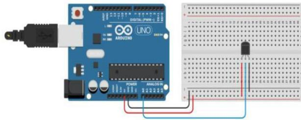
**Figure 7. Temperature Sensor LM35**
