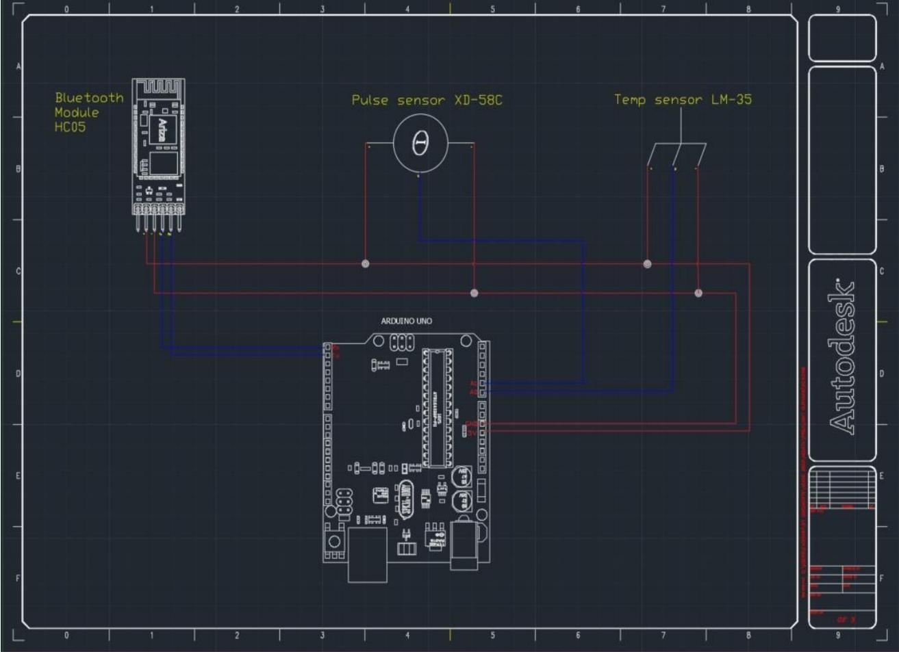
**Figure 9: Overall Hardware Design**
