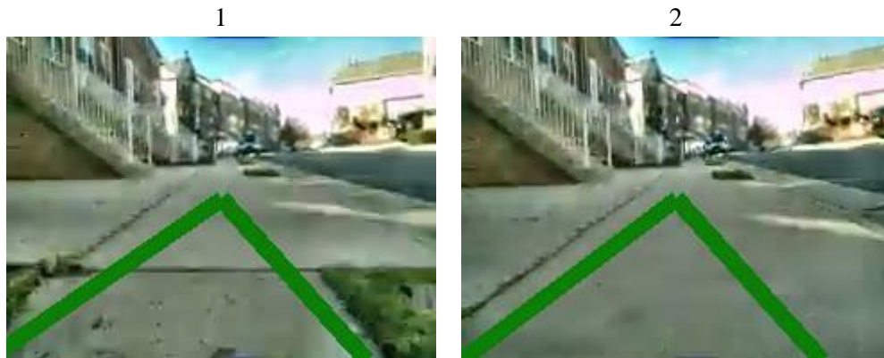
Figure 39. Annotations and context. In the first image it is understandable why the annotation is done like it. In the next image it is not so obvious. If there is no context then it is not understandable why the pavement width is marked so narrow.
