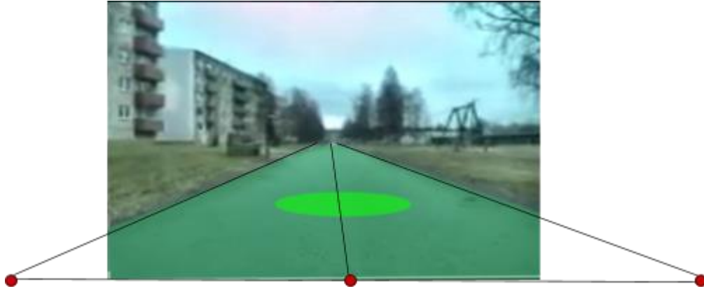
Figure 14. Calculating intersection points. The red points are calculated from current annotations. Right and left red points with the image are given to the algorithm as inputs.
