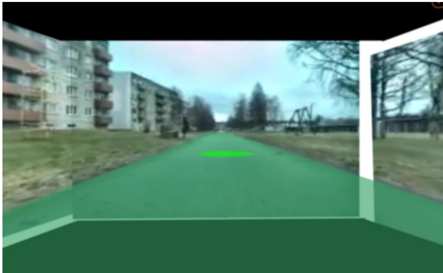
Figure 12. Image while 3D mapping. The centre camera and side cameras are put together. The green area marks the pavement and the yellow represents a node.
