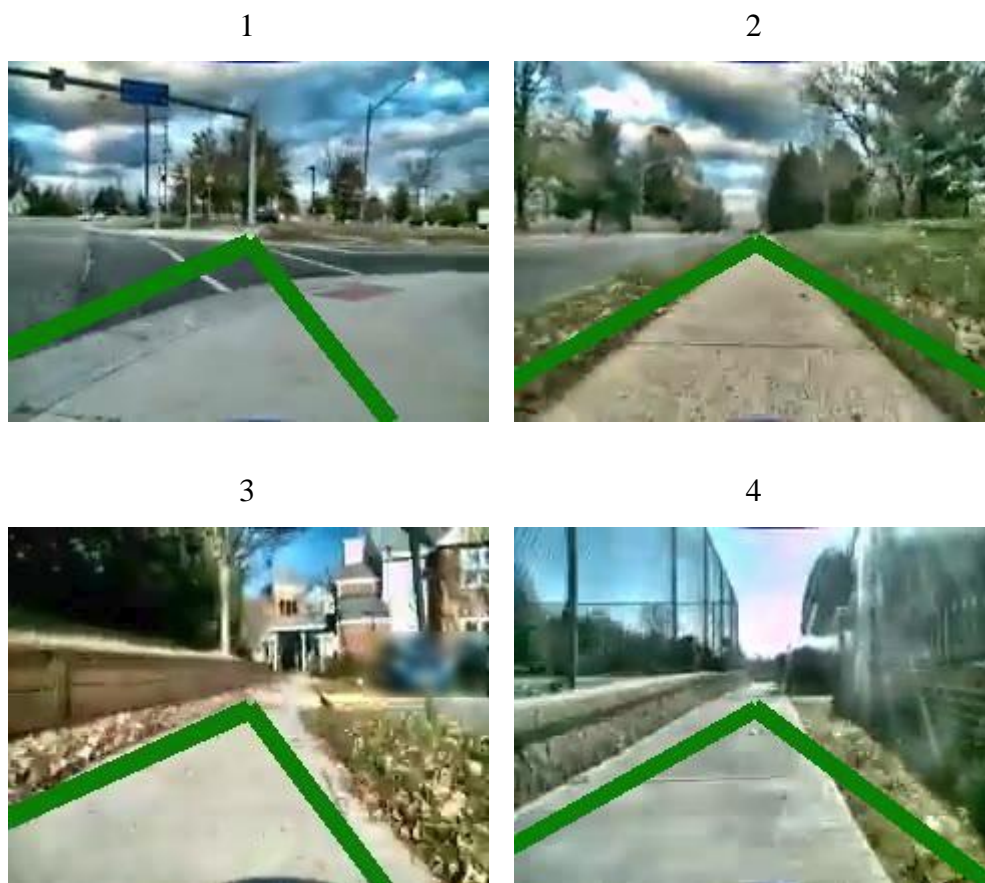
Figure 38. Bad input examples. The green lines are drawn from the intersection points to the image centre. 1) Not the whole pavement mapped. 2) Marked too wide. 3) Not marked whole pavement. 4) Marked too wide.
