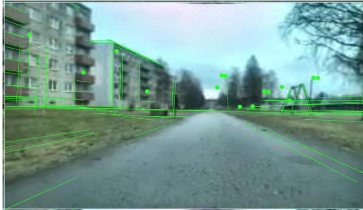
Figure 2. Localisation map. The map consists of lines that robot sees around it in a certain location. The green lines in the picture are mapped lines and the dots are mapped light sources used for night-time navigation.
