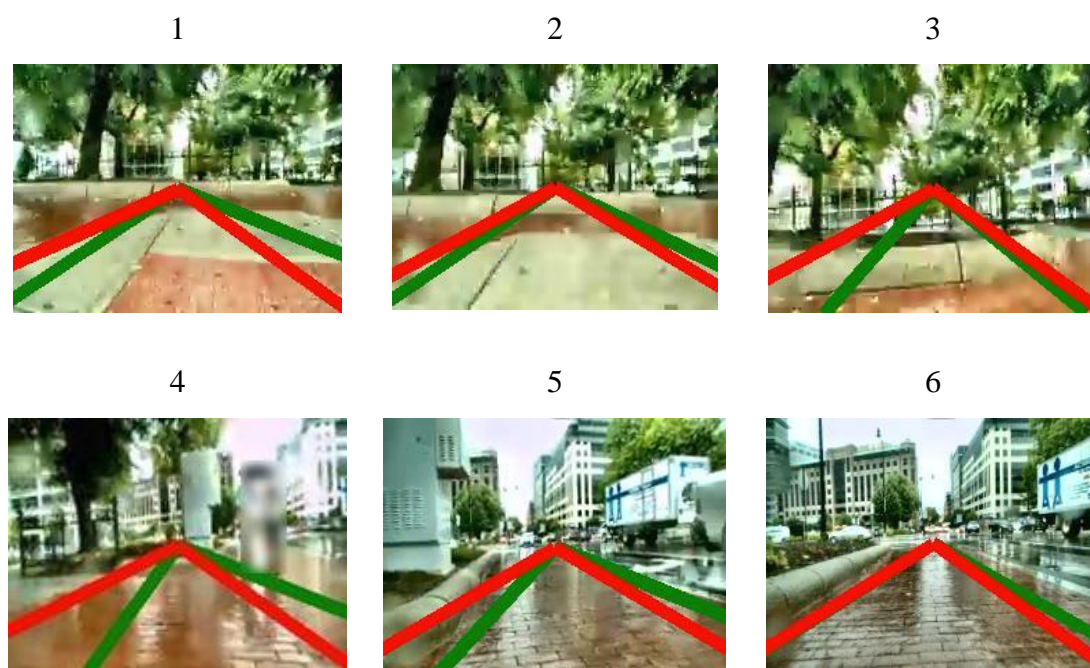
Figure 40. Images algorithm struggles with. Red lines are from neural network model predictions to the image centre and the green are training data points to image centre. The image number 6 is correct after all the curb climbing and turning corner, but it can be seen from the images that the curb climbing (1, 2) and turning (3, 4, 5) might not be so accurate.
