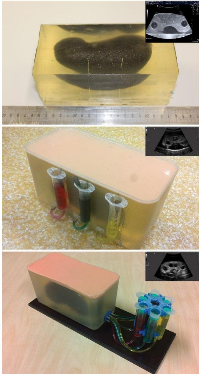
*Figure 3.2 Different versions of kidney phantoms used in the interventional radiology training (upper image: simple kidney phantom with puncturing targets made from clear gelatin; middle image: kidney phantom with three drainable calyces; lower image: kidney phantom with six calyces connected to outer reservoirs with hoses aligned under the kidney as a descending ureter)*
