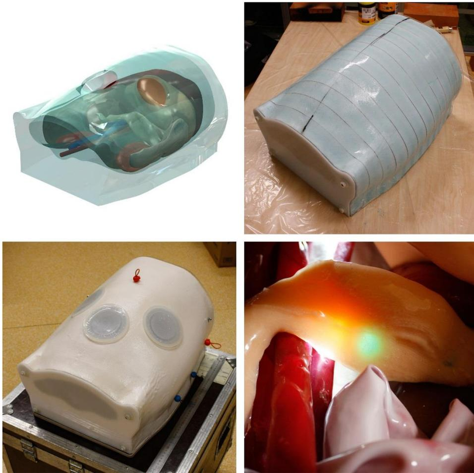
*Figure 2.2 Pig abdominal phantom (from upper left to lower right: model of the abdomen reconstructed from CT; Styrofoam model of the abdomen covered with glass fiber, painted and assembled abdomen; view to the silicon pancreas through the middle port)*
