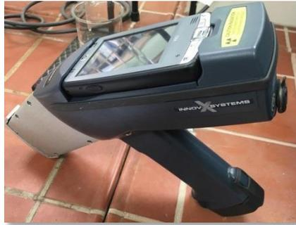
Fig 2.6. Innov-x Systems Hand XRF
