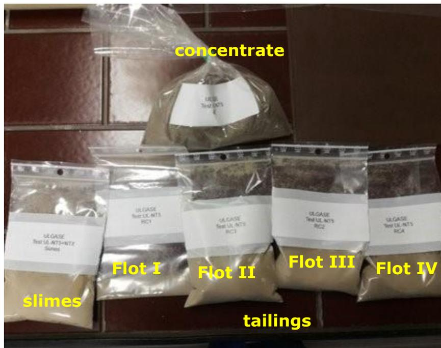
Fig 2.2. Final Samples collected from the flotation process
