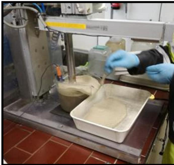
Fig.5 The float collection (visually the main component is silica)
