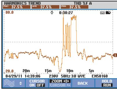
Fig. 15. Total harmonic distortion of the capacitor current, during some interval the  $THD_u$  reaches 80%.
