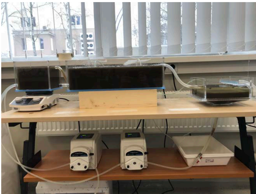
Figure 3.6 APAC test where PAC was dosed into the first, anoxic reactor.
