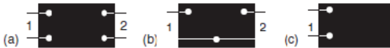
Fig. 1.1. Black boxes. The two boxes (a) and (b) allow for transfer parameters from one port to the other. Box (c) is a one-port, two-terminal box with only driving point parameters possible.
