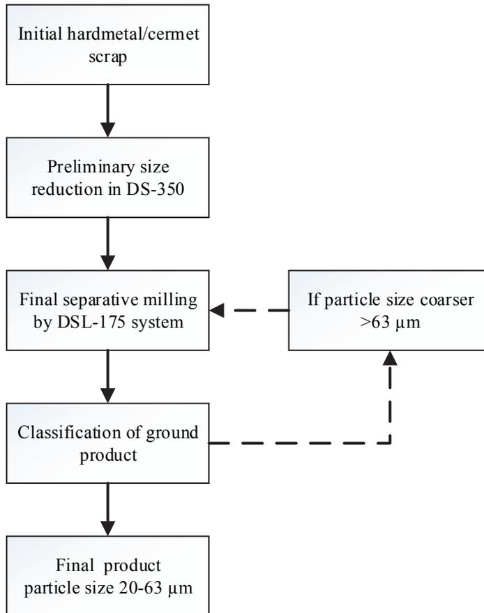
Figure 2.3 Work procedure of retreatment of hardmetal/cermet scrap
