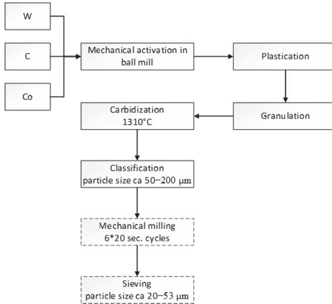
**Fig.1:** Powder production process via mechanically activated synthesis
