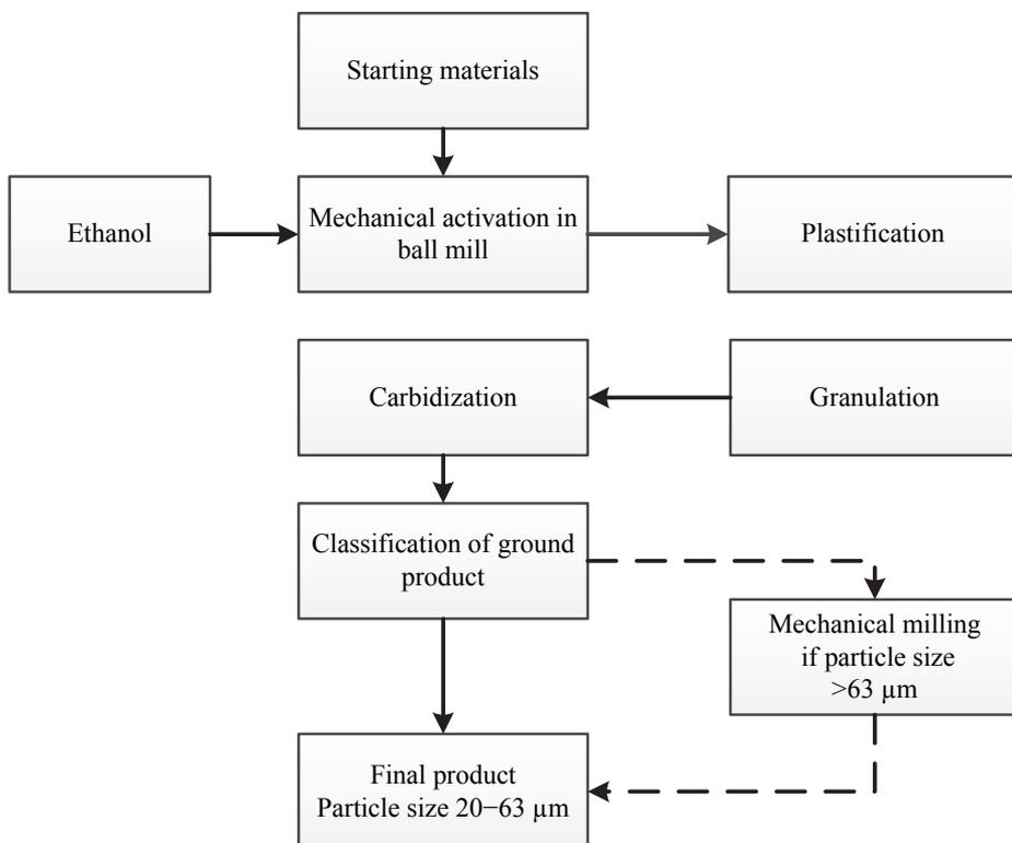
Figure 2.1 Principal scheme of the mechanically activated thermal synthesis [Paper I and Paper IV]
