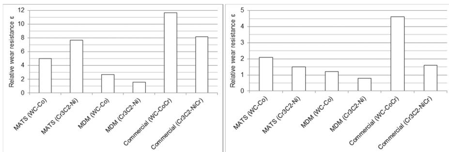
Figure 3.9 Potential application areas of HVOF sprayed coatings based on wear resistance at different applications: a – at ARWW; b – at AEW (30°).
