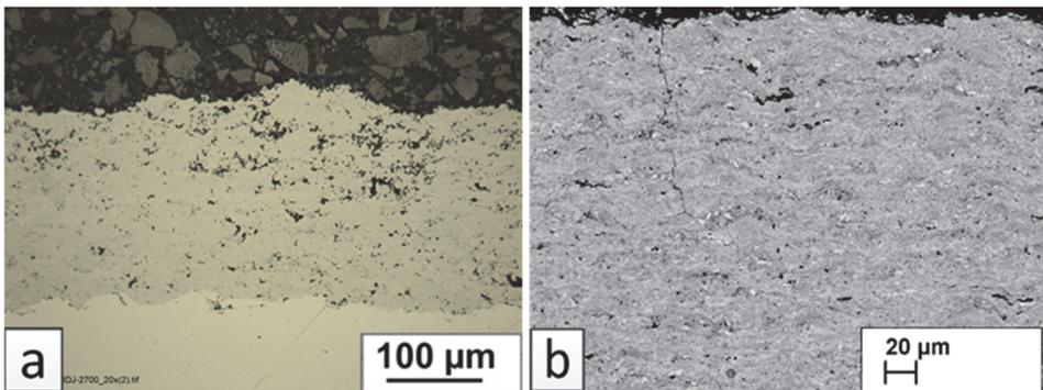
Figure 3.3 Microstructure of HVOF sprayed coatings from commercial spray powders: a – WC-CoCr (Amperit 558); b – Cr<sub>3</sub>C<sub>2</sub>-NiCr (Amperit 588)
