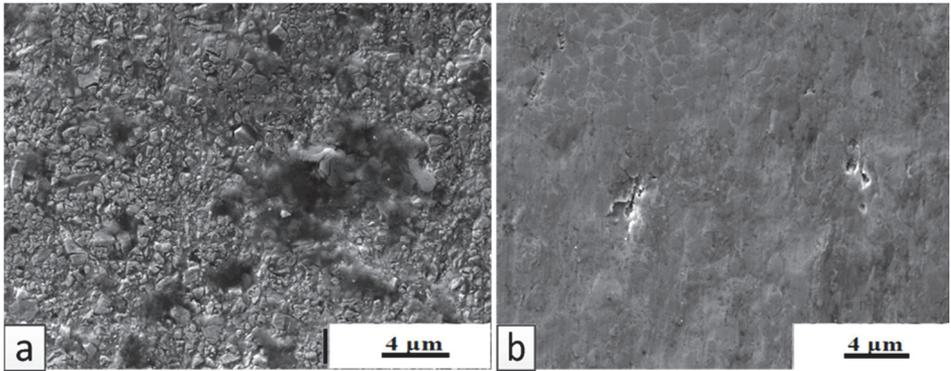
Figure 3.5 Topography of worn surfaces at ARWW of sprayed coatings from MATS hardmetal/cermet powders: a – WC-Co; b – Cr<sub>3</sub>C<sub>2</sub>-Ni
