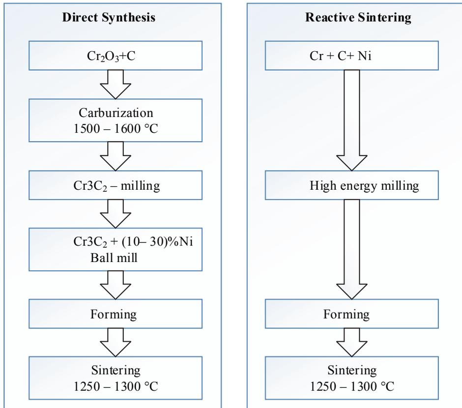
Figure 1.2 Production of chromium cermets based carbides [Pirso, 2006]
