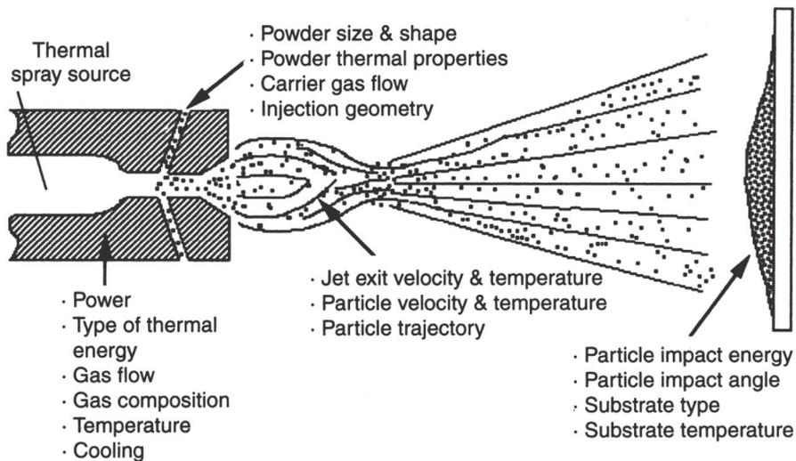
Figure 1.5 Variables and parameters of a typical thermal spray process [Gan, 2015]
