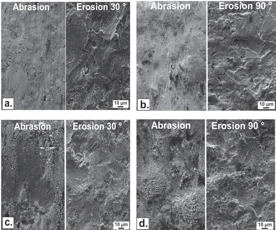
**Fig. 5.** Worn surfaces of the coatings after abrasive wear: a – (Cr<sub>3</sub>C<sub>2</sub>-Ni)+ FeCrSiB; b – (Cr<sub>3</sub>C<sub>2</sub>-Ni)+ NiCrSiB; c – (WC-Co)+ FeCrSiB; d – (WC-Co)+ NiCrSiB
