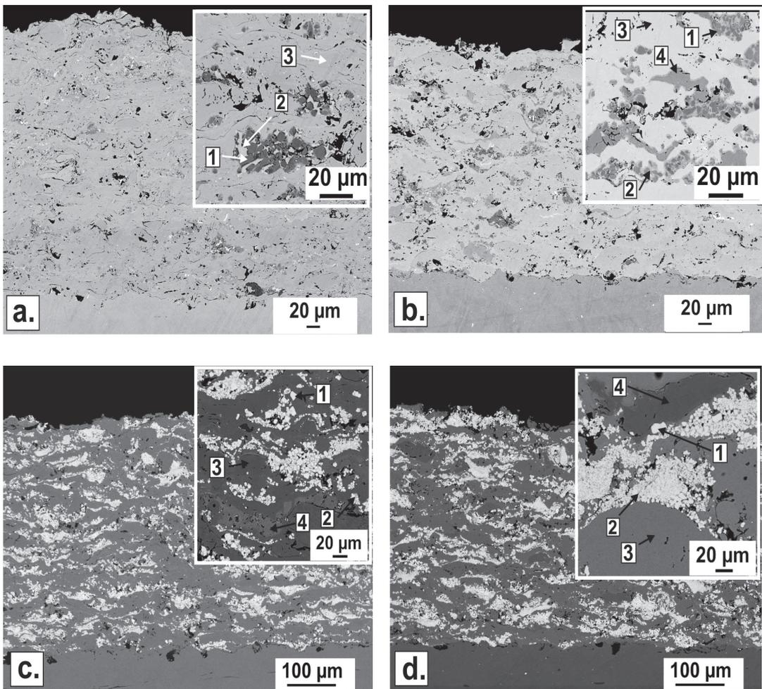
**Fig. 4.** Coatings cross-sections and EDS phasemaps (window areas): a –  $(\text{Cr}_3\text{C}_2\text{-Ni})+\text{FeCrSiB}$ ; b –  $(\text{Cr}_3\text{C}_2\text{-Ni})+\text{NiCrSiB}$ ; c –  $(\text{WC-Co})+\text{FeCrSiB}$ ; d)– $(\text{WC-Co})+\text{NiCrSiB}$
