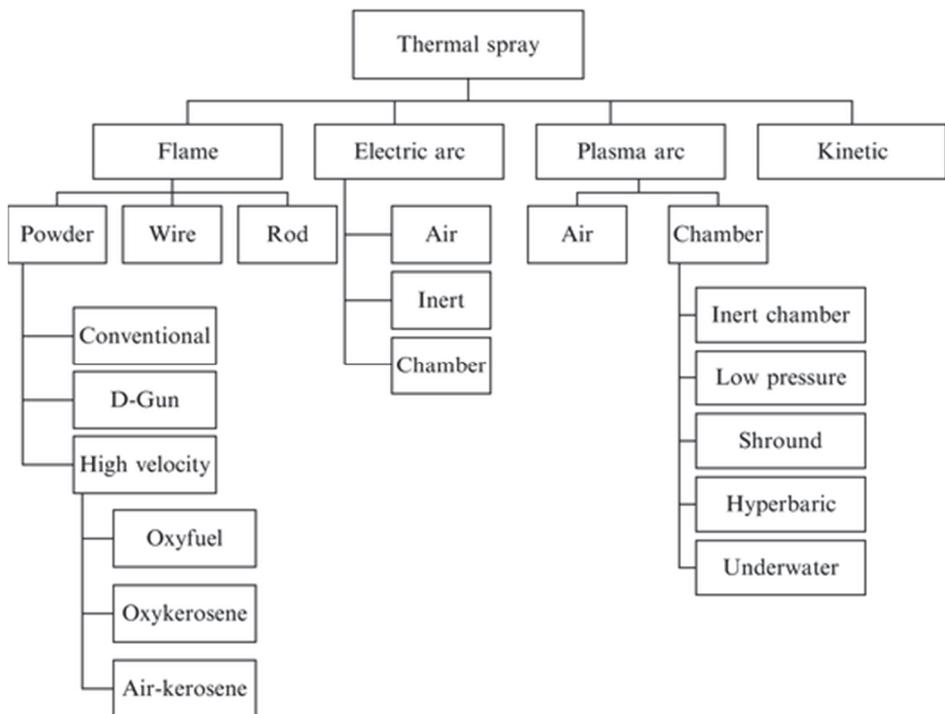
Figure 1.4 Classification of thermal spray processes and subsets [Majumdar, 2014]
