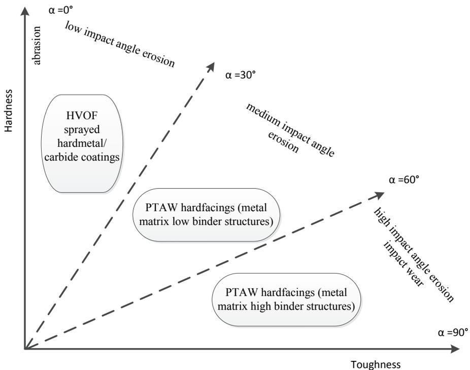
Figure 3.10 Potential application areas of sprayed coatings (for comparison PTA-welded hardfacings)
