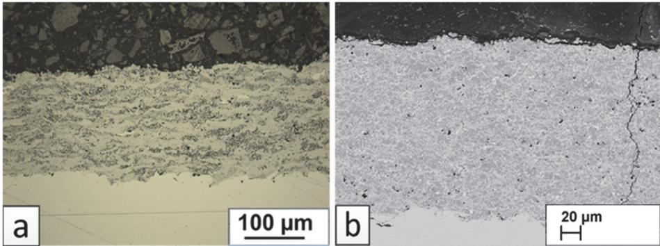
Figure 3.2 Microstructure of HVOF sprayed coatings from experimental MATS powders: a – WC-Co; b – Cr<sub>3</sub>C<sub>2</sub>-Ni
