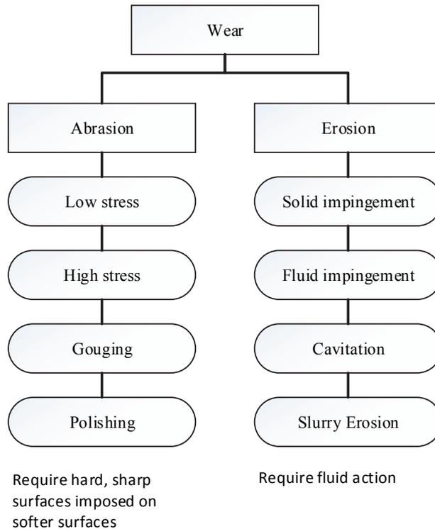
Figure 1.9 Major categories of wear based on abrasion and erosion [Veinthal, 2011]
