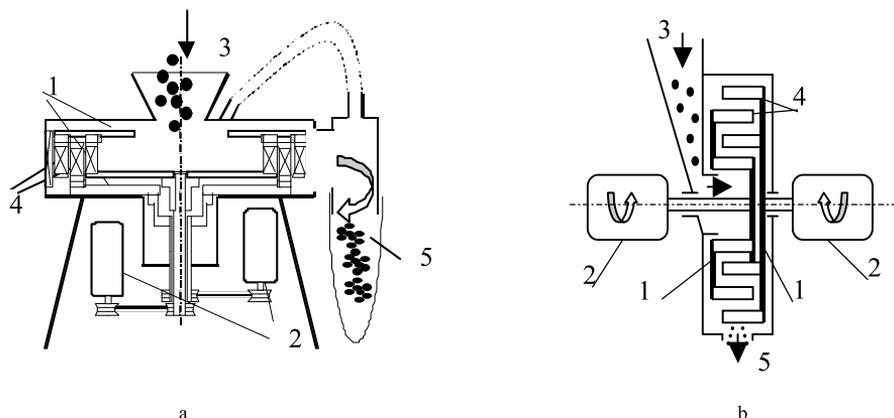
**Fig. 1.** Schematic representation of preliminary size reduction centrifugal-type mill DSL-350 (a) and vertical laboratory milling disintegrator DSL-175. Equipment (b): 1 – rotors; 2 – electric drives; 3 – material supply; 4 – grinding elements; 5 – output
