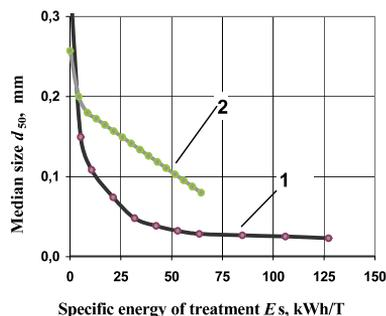
**Fig. 3.** Dependence of the median particle size  $d_{50}$  on the specific energy of final multi-stage milling. Grindability curves of materials: 1 – ( $\text{Cr}_3\text{C}_2\text{-Ni}$ ); 2 – ( $\text{WC-Co}$ )
