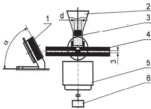
**Fig. 3.** Principal scheme of block-on-ring wear tester: 1 – specimen; 2 – abrasive particles vessel; 3 – shield; 4 – rotor; 5 – drive motor; 6 – rotation frequency gauge
