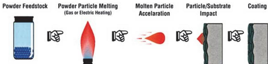
Figure 1.8 Flowchart of HVOF spray process [AWS, 2015]
