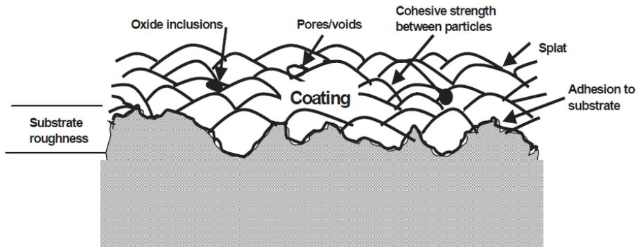
Figure 1.6 Typical cross-section of a thermal sprayed coating [Engineering Manual EM 1110-2-3401, 1999]
