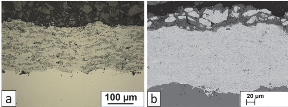
Figure 3.4 Microstructure of HVOF sprayed coatings from commercial self-fluxing alloy and MDM hardmetal/cermet mixtures: a – FeCrSiB+(WC-Co); b – FeCrSiB+(Cr<sub>3</sub>C<sub>2</sub>-Ni)
