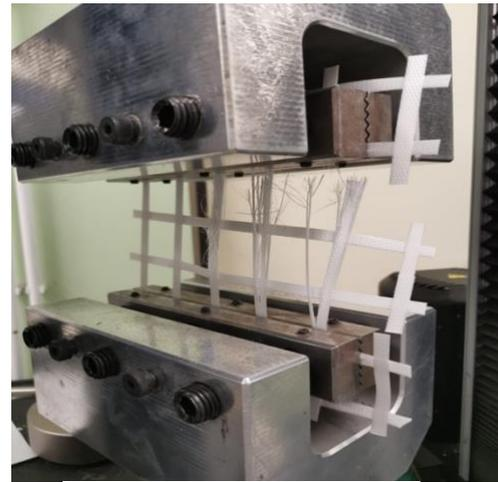
Tensile strength test of PP
