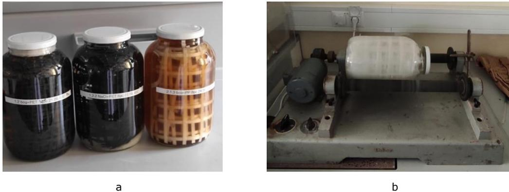
Figure 1.9 Positioning and mixing of specimen in two stages (a) specimen in solution and (b) homogenization
