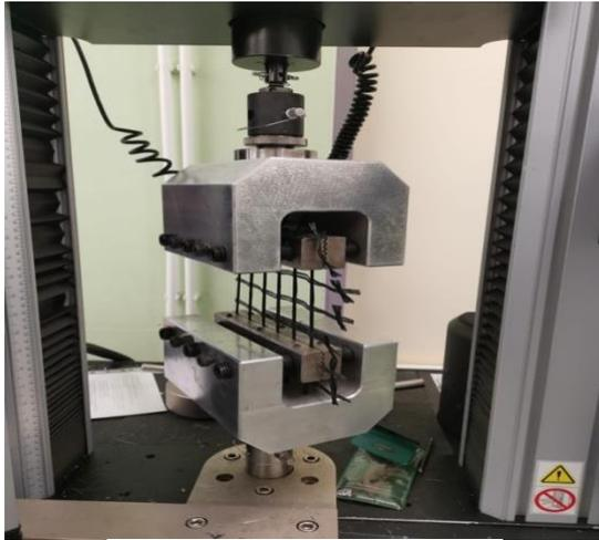
Tensile strength test of PET
