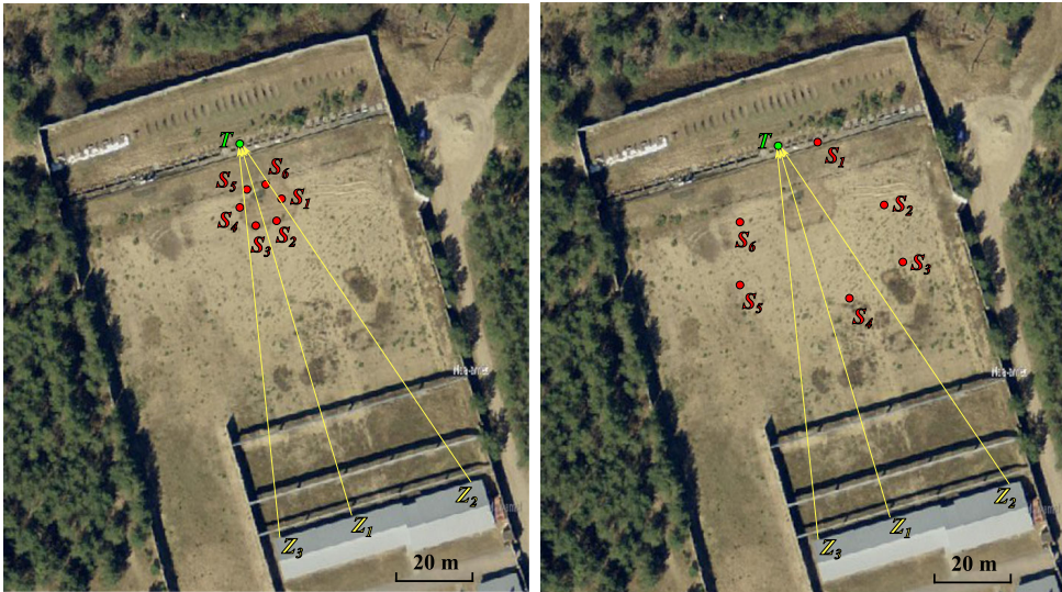
Fig. 11 Layout of Experiments 2 (left) and 3 (right). T –target position; Z_i –shooter positions; S_k –UGS positions
