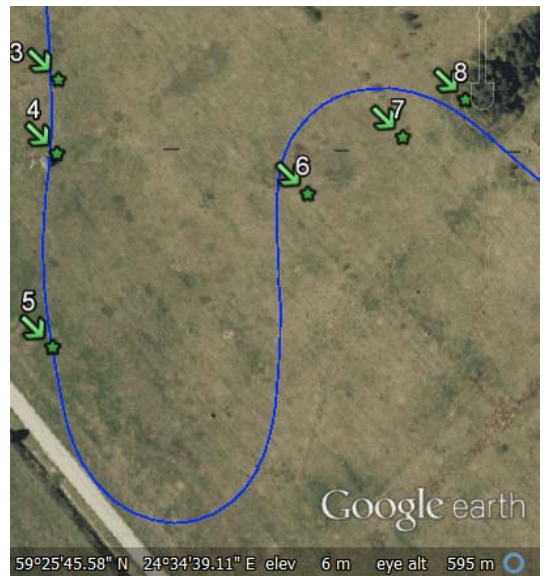
Fig. 11. UAS flight path in case of two consecutive subscriptions involving targets very close to eachother (targets are at wp-s 4 and 8, rest of the waypoints are generated for UAS guidance).
