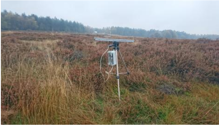
Figure 3 – WSN microphone array sensor. The linear array itself consists of 6 microphones, the distance between each microphone is 10 centimetres.
