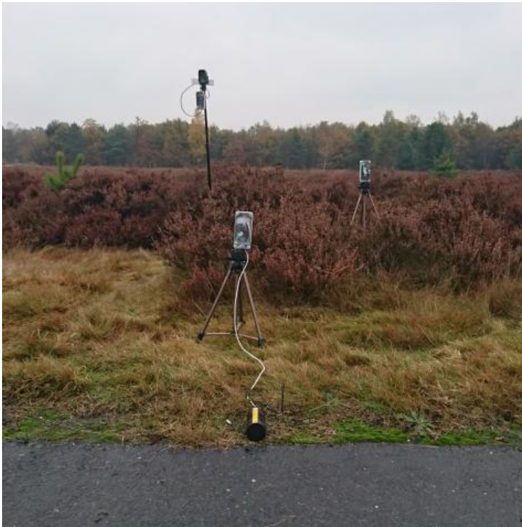
Figure 4 – WSN sensor set consisting of a motion detector, magnetic field change detector and a video based moving object counter.
