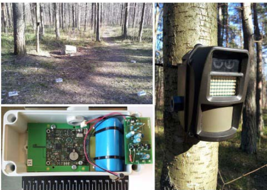
Fig. 3. Defendec Smartdec device on the right, experimental magnetic field sensor on the bottom left and experimental sensors in the forest in the left top
