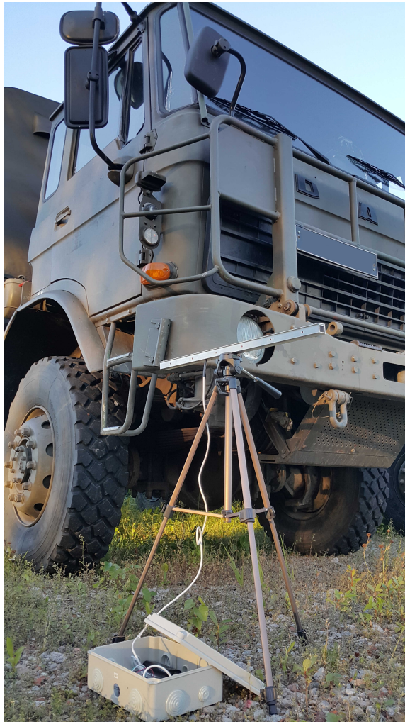
Figure 32 - An acoustic sensor node with vehicle used in experiment.
