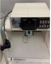
Figure 9. CE-LED-induced fluorescence detector (TUT and LDI AS, Estonia)
