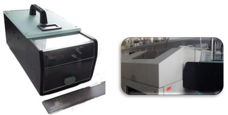
Figure 10 In-house built portable CE device coupled to C<sup>4</sup>D (TUT, Estonia)
