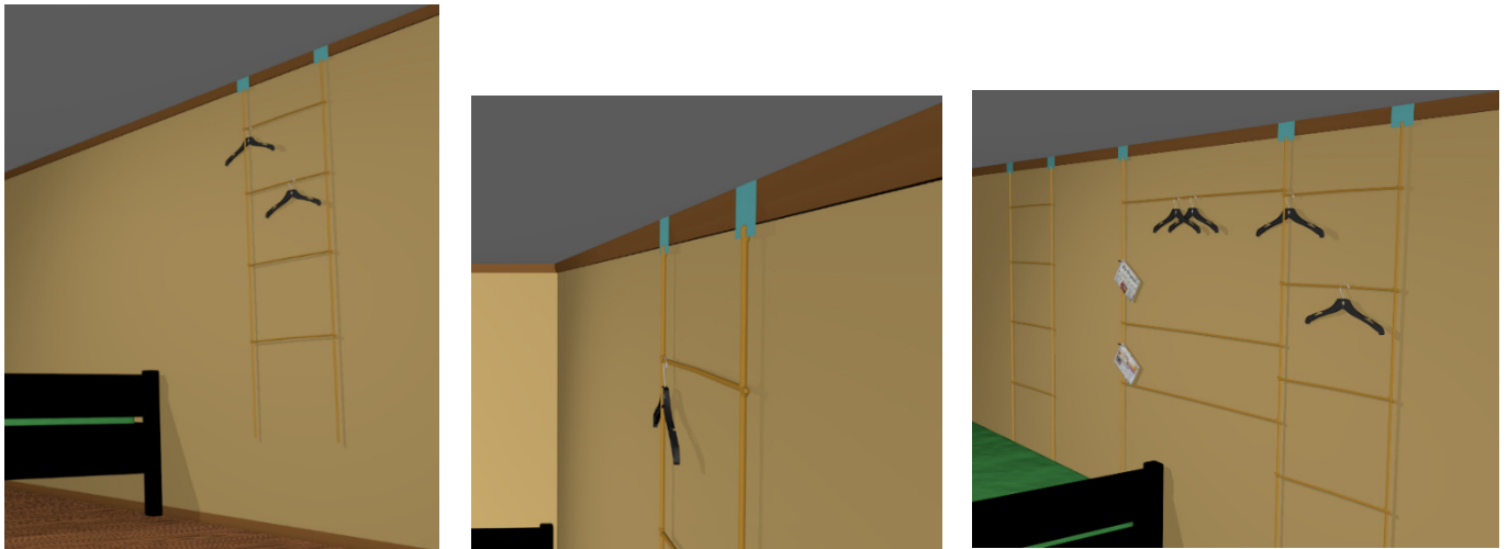
Figure 18 Concept model of storage system hung from mouldings
