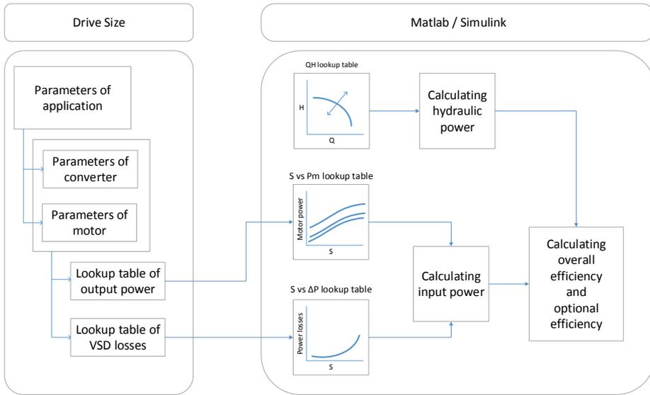
Fig. 3.13 Architecture for simulation the multi-drive multi-pump station.
