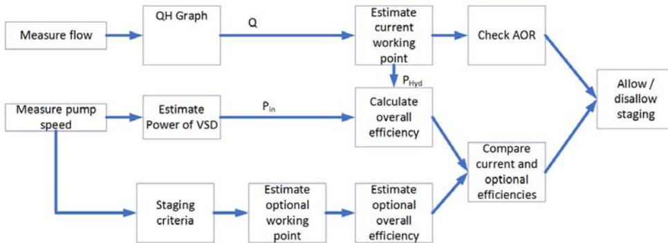
Fig. 3.7. Program architecture for implementation of the efficiency-based control method on a PLC platform.
