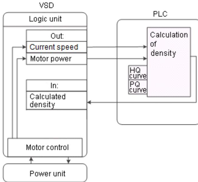
Fig. 4.9. Data flow between the VSD and the PLC.
