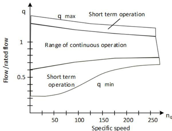
*Fig. 3.2 Recommended ranges for continuous and short-term operation regarding the flow (Gülich, 2008).*
