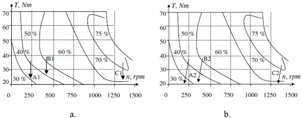
Fig. 4.12 Efficiency maps of an induction motor in the torque-speed reference frame. The source data are taken from (P. Angers, 2009). The arrows indicate an efficiency change after the torque drop for stable speed case (a) and 10% speed inaccuracy case (b).
