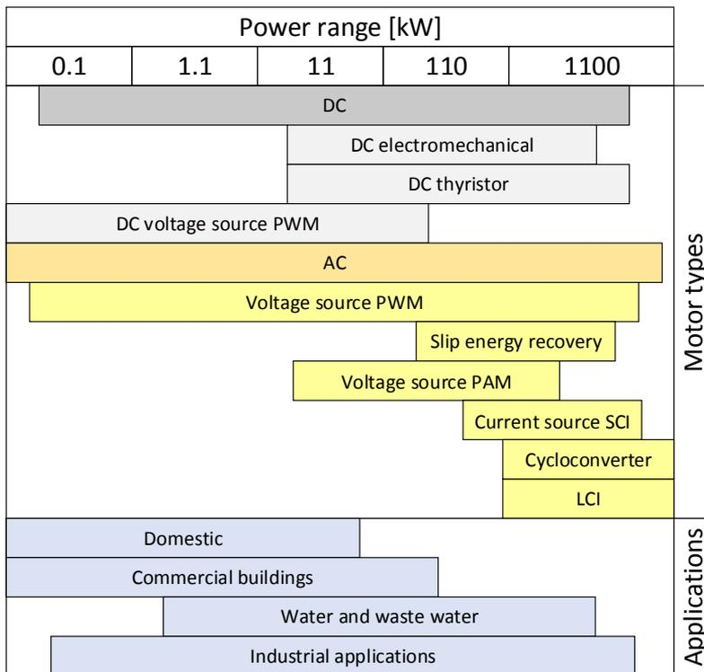
Fig. 1.11 Application fields and power ranges for VSDs.
