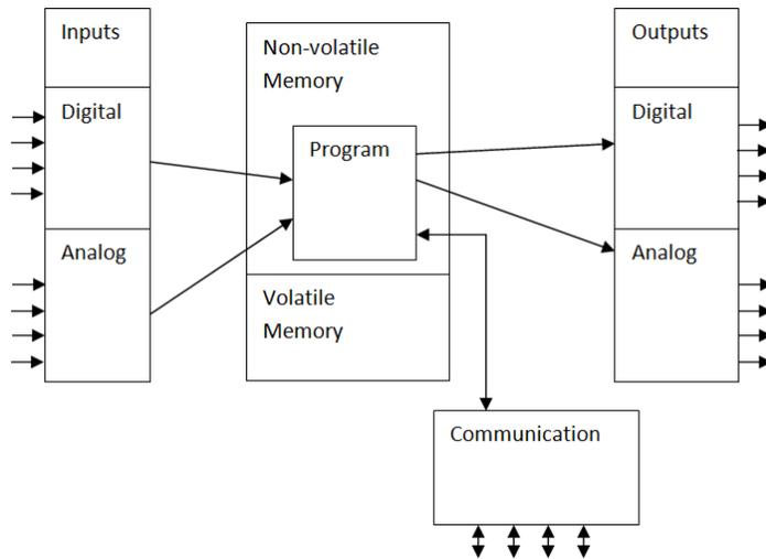
*Fig. 2.9 Simplified diagram of the PLC.*
