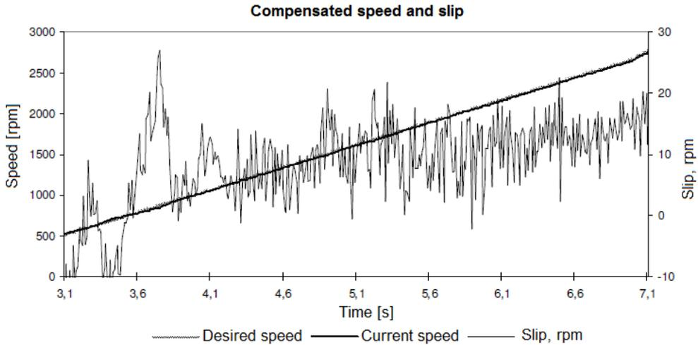
Fig. 4.16 Logged readings of slip and speed under the proposed compensation method.
