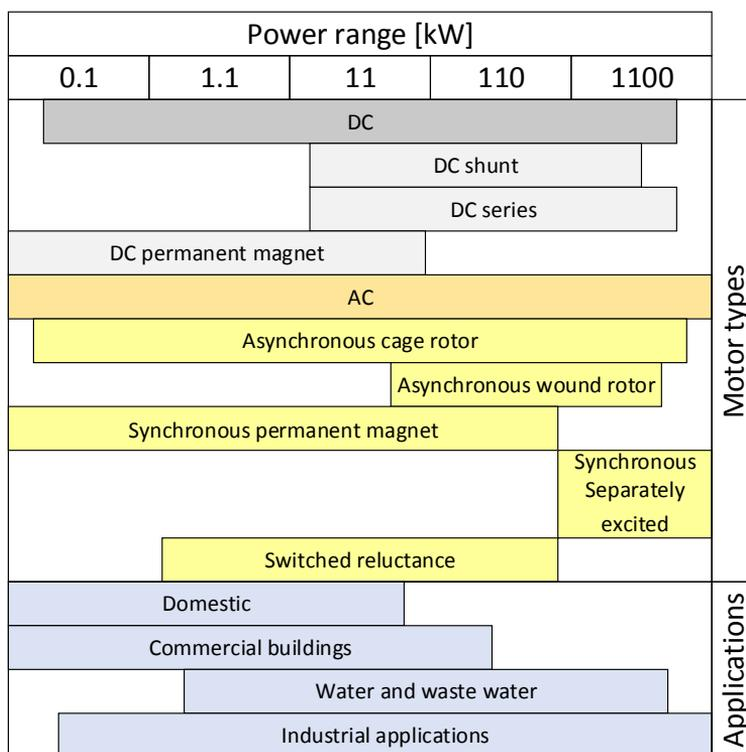
Fig. 1.10 Application fields of different motor types in pumping applications.
