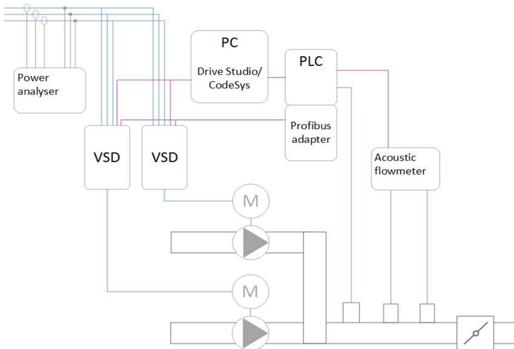
Fig. 3.17 General diagram of the test stand.
