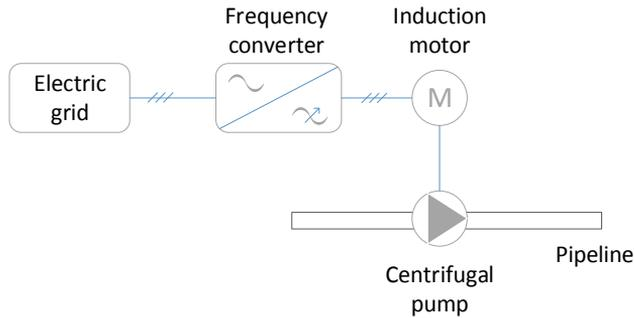
Fig. 1.12 Typical single-pump pumping system.
