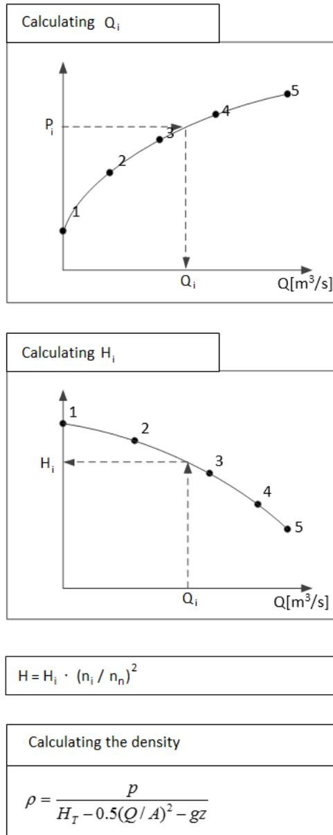
Fig. 4.8 Algorithm of density calculation.
