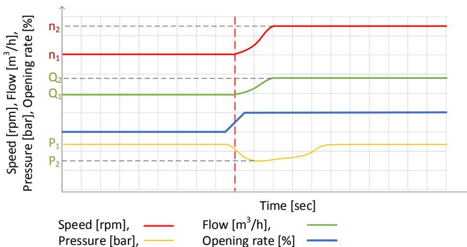
Fig. 1.6 Dynamics of pumping parameters at an increase of piping system conductivity.
