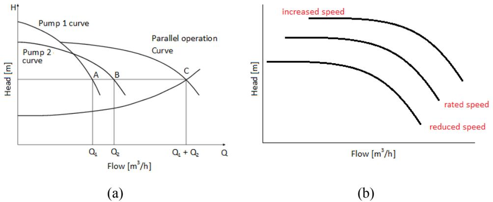
Fig. 3.10. Parallel operation of two pumps (working points A and B). The combined curve and resulting operating point location C with the total flow rate  $Q_1 + Q_2$  (a) (Bortoni, 2008) and shifting correspondingly to speed dynamics (b).
