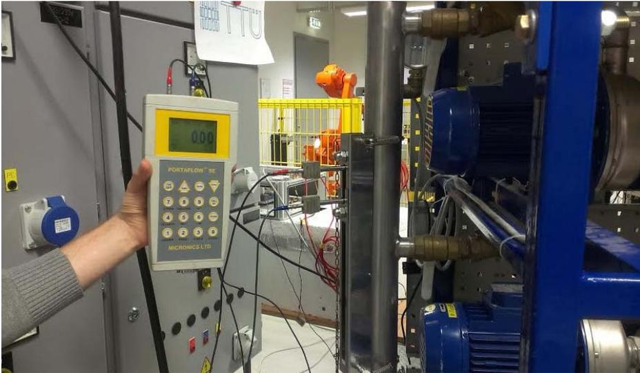
*Fig. 2.11. PORTAFLOW™ SE in the test stand.*
