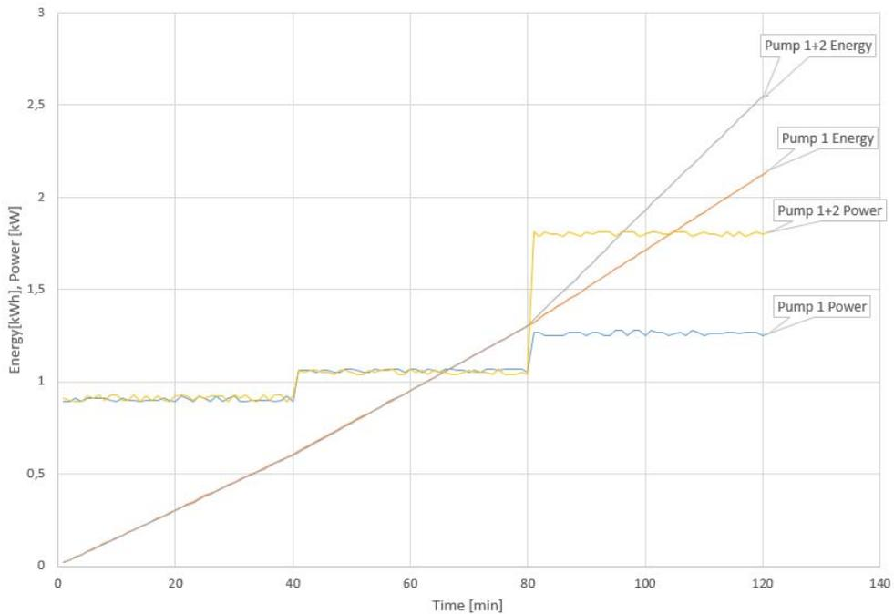
Fig. 3.19 Energy consumption of the experimental pumping system
