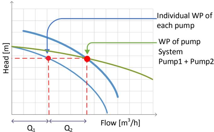
Fig. 1.9 Combined and individual HQ curves for pumping system when two pumps are running.
