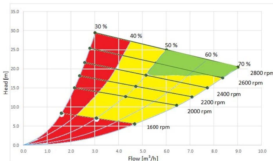
Fig. 1.18 Operating regions mapped on the HQ characteristic graph of Ebara 120/12 pump: recommendable (green), allowable (yellow), and avoidable (red).
