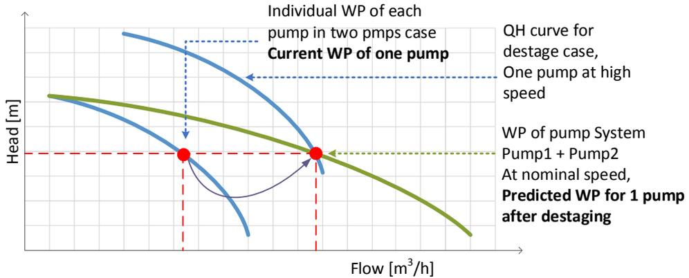
Fig. 3.9 Graphical representation of the predicted state for the destage case.
