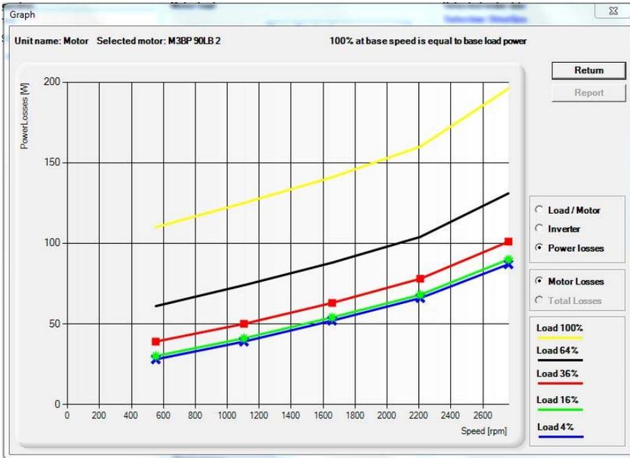
Fig. 2.5 Characteristics for obtaining the power losses of VSD. The graph is generated by the DriveSize tool.
