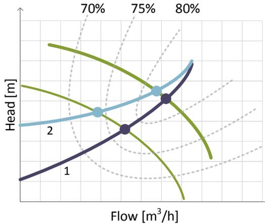
Fig. 1.14 Displacement of the working point of a pump as a result of varying rotational speed: 1 – for low static head, 2 – for high static head.
