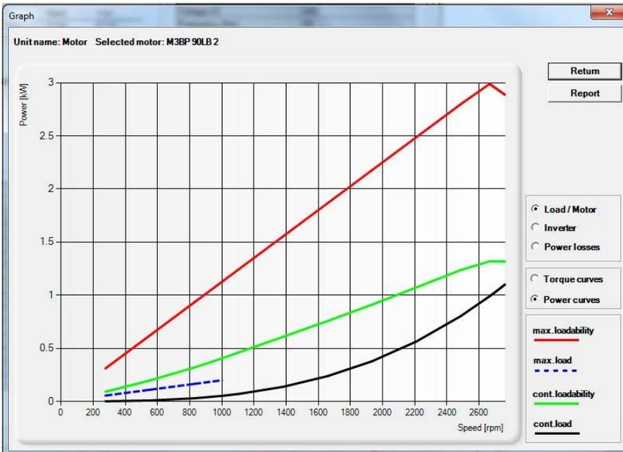
Fig. 2.6 Characteristics for obtaining the motor current power. The graph is generated by the DriveSize tool.
