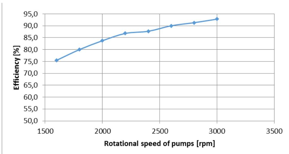
Fig. 1.17 Efficiency of 1.1 kW frequency converter (ACQ810-04-02A7-4) running the motor and the centrifugal pump (EBARA 120/12).
