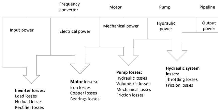
Fig. 1.13 Types of power losses in a pumping system.
