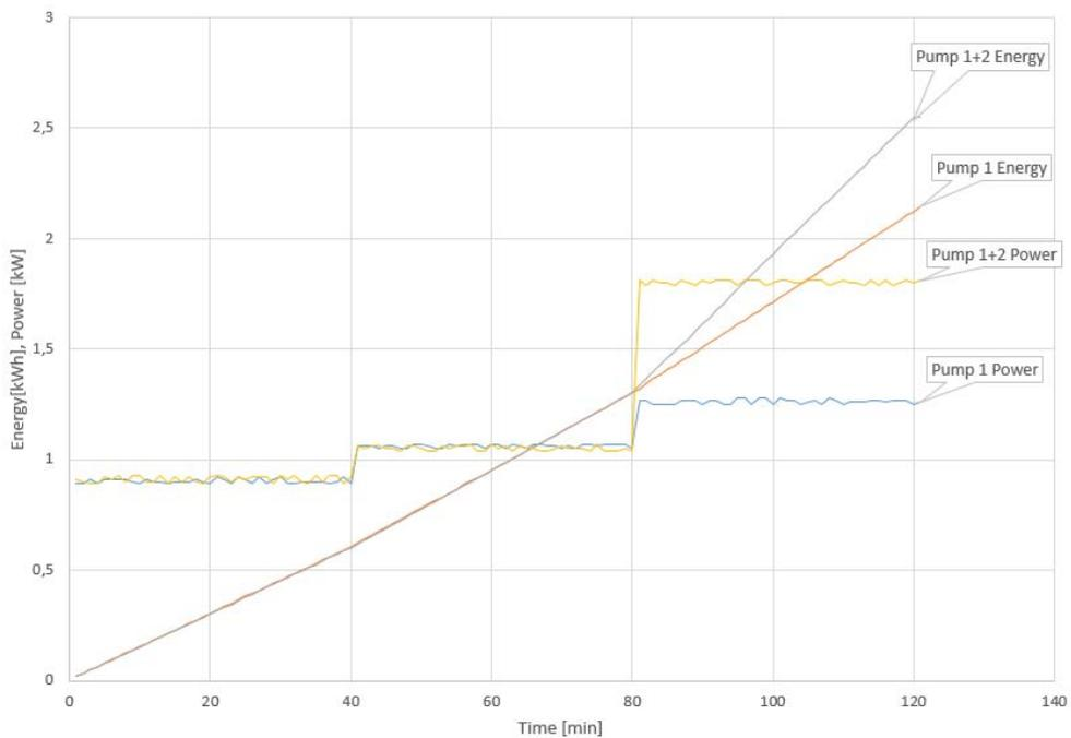
Fig. 3.19 Energy consumption of the experimental pumping system
