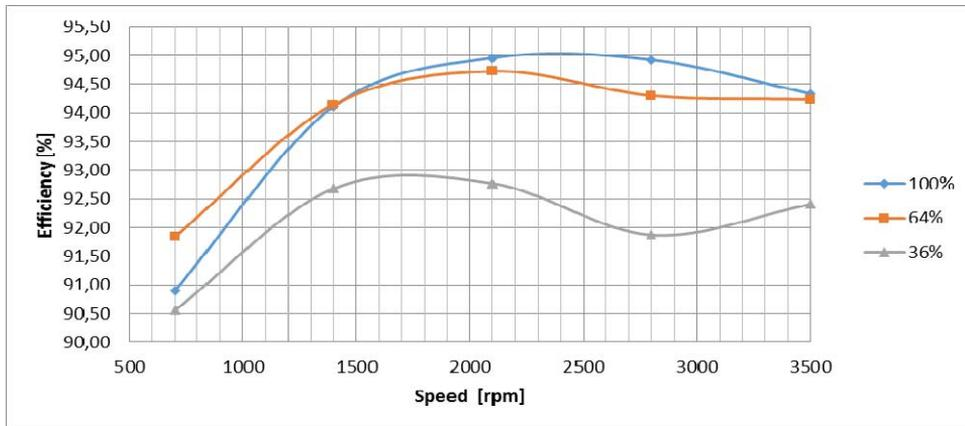
Fig. 1.16 Motor efficiency vs. speed of 18.5kW, 95 % efficient motor, M3BP 160MLC 2, ABB.
