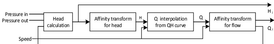
Fig. 3.6. Steps of the HQ graph based estimation method (Ahonen, 2011).
