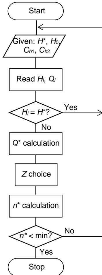
Fig. 3.12 Control algorithm.
