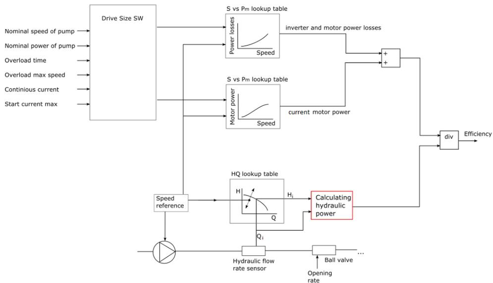
Fig. 2.2 Diagram of a model providing efficiency calculations.
