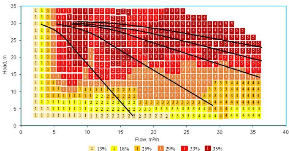
Fig. 3.4 Efficiency map for five parallel connected pumps Ebara CDX 120/12.
