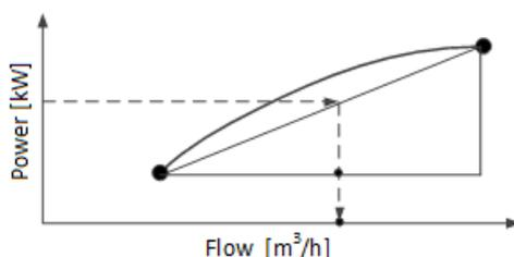
Fig. 4.7 Interpolation method using the triangles similarity rule.
