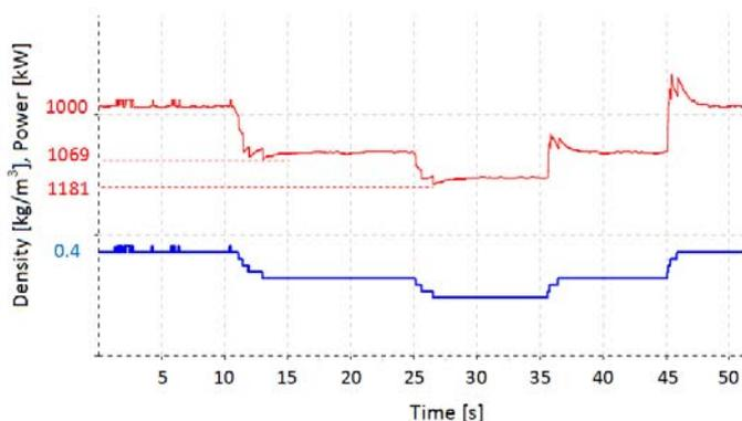
Fig. 4.11 Measuring the density. Simulating the density change by increase / decrease of the tested pump loading.
