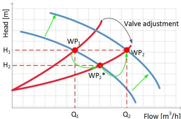
Fig. 1.5 Rotational speed of a pump increases making the HQ curve shift up and to the right.  $WP_2^*$  is a transitional point.
