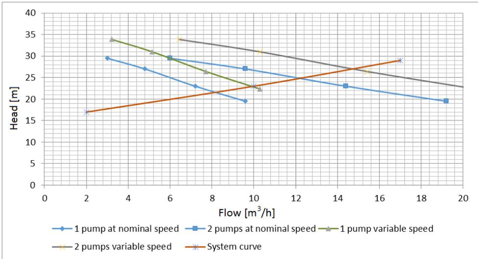
Fig. 3.14 Pump characteristic curves for 1 pump and 2 pumps cases. The graph shows that the flow of 8 m<sup>3</sup>/h can be provided by 1 pump running at 2800 rpm or by 2 pumps when each is running at 2500 rpm (the intersection of HQ curves with the system curve at 8 m<sup>3</sup>/h).
