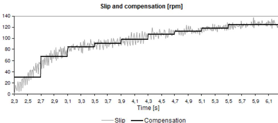
Fig. 4.14 Compensating the slip with compensation values from the lookup table.
