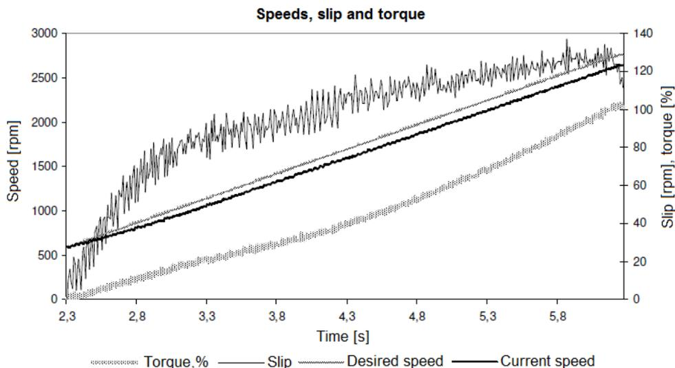
Fig. 4.13 Accelerating a pump during the tuning stage.
