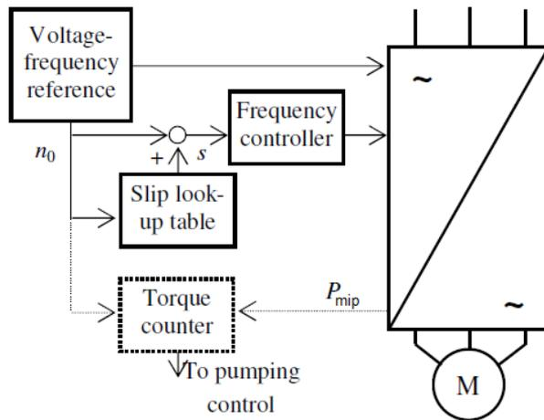
Fig. 4.15 Diagram of the sensorless slip compensation.  $P_{mip}$  is motor input power.
