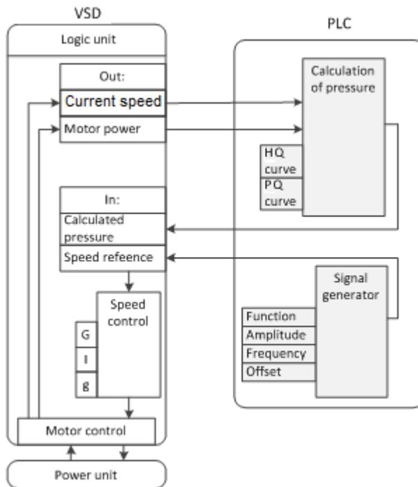
Fig. 4.2 Data flow between the PLC and the control unit of frequency converter.
