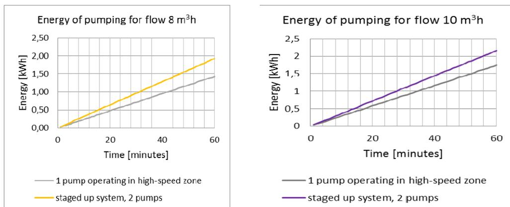
Fig. 3.16 Energy consumption of pumping system providing flow of 10 m<sup>3</sup>/h and 8 m<sup>3</sup>/h.
