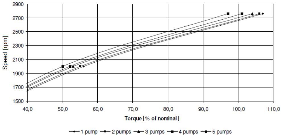
Fig. 4.17 Speed-torque characteristics of five pumps Ebara CDX 120/12.
