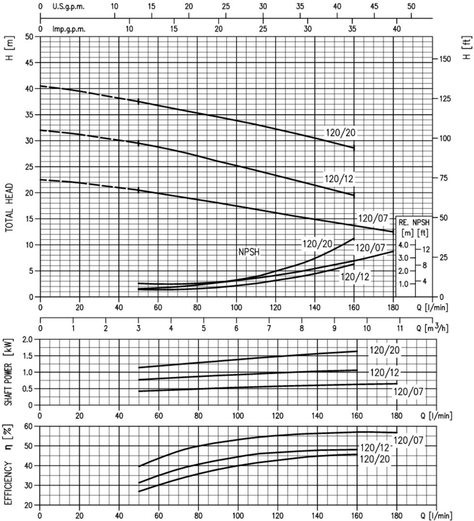
Fig. 1.2 Characteristic curves of an Ebara CDX 120 series pump provided in the datasheet.
