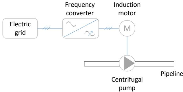
Fig. 1.12 Typical single-pump pumping system.
