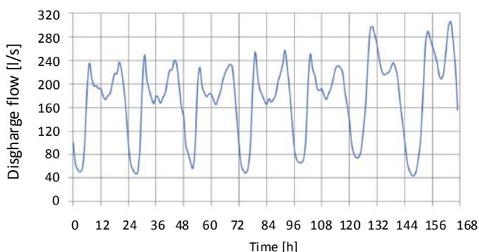
*Fig. 1.4 Weekly graph of a discharge flow at “Punane” pumping station in Tallinn.*
