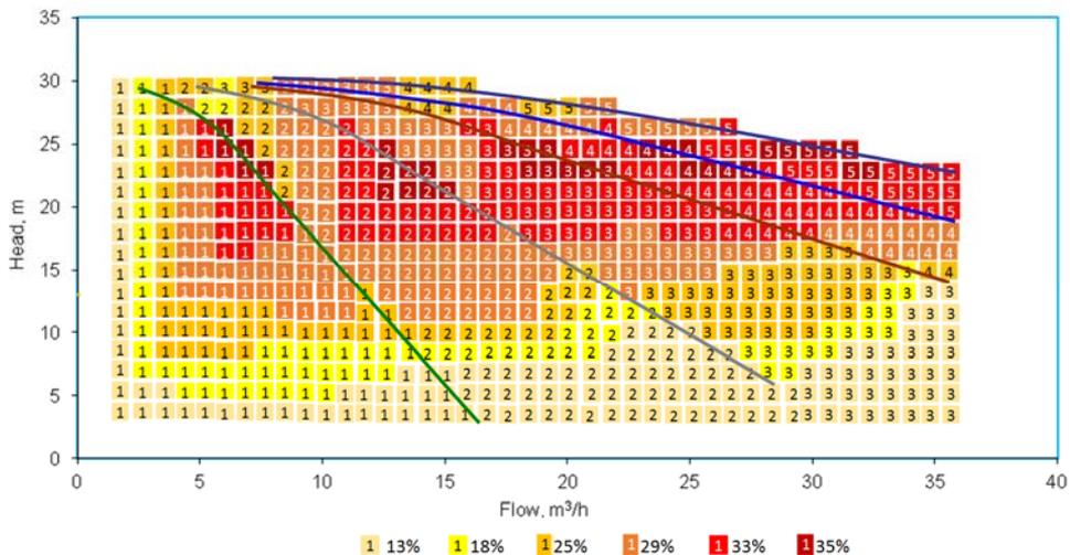
Fig. 3.5 Efficiency map for the traditional speed-oriented approach.
