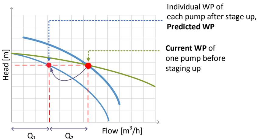
Fig. 3.8. Graphical representation of the predicted state for the staging up.
