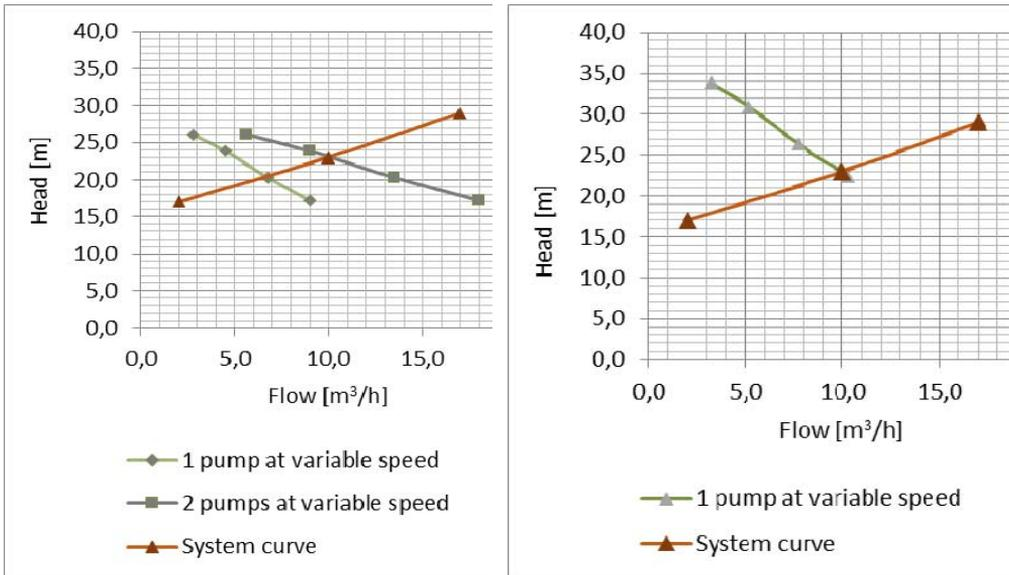
Fig. 3.15 HQ characteristic curves for providing 10 m<sup>3</sup>/h in high-speed case (right) and staged up case (left).
