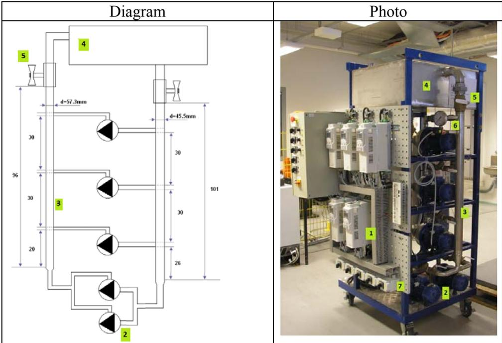
*Fig. 2.7 Experimental setup: 1 – frequency converter; 2 – centrifugal pump; 3 – pipeline; 4 – water tank; 5 - main valve; 6 – digital and analogue pressure sensors; 7 – switches for switching between the variable-speed and direct power supply modes.*
