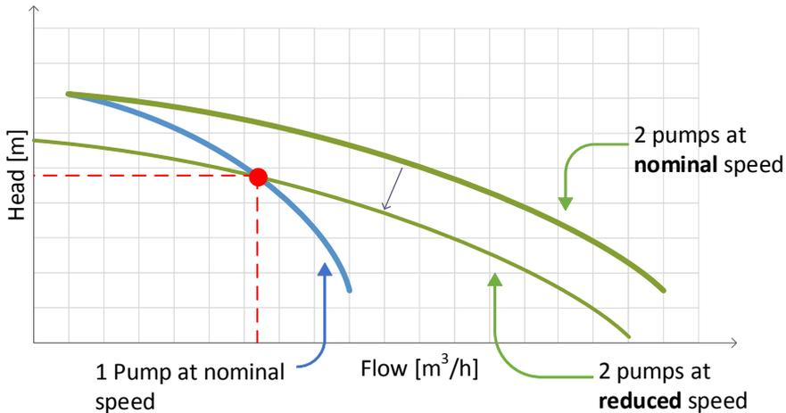
*Fig. 1.8 Two options of keeping the pumping system at the working point: using one pump or two pumps at reduced speed.*
