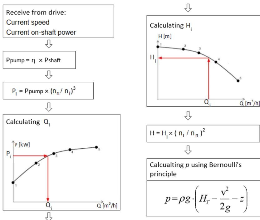
Fig 4.1 Algorithm of pressure estimation implemented in the PLC.
