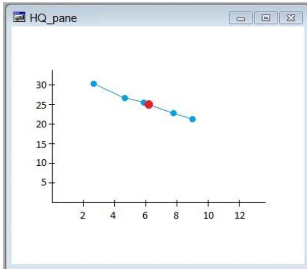
*Fig. 2.10 CodeSys visualization panel showing the current location of the working point at 6 m<sup>3</sup>/h.*
