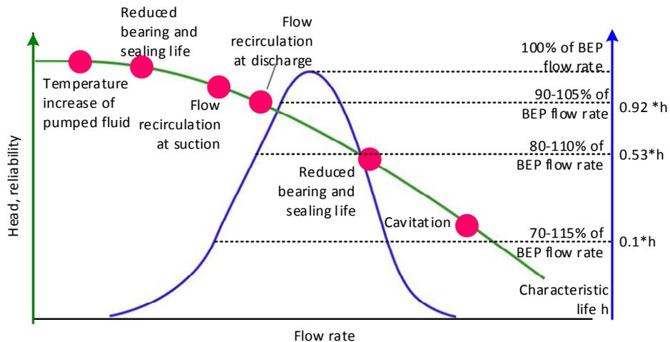
Fig. 3.1 Pump reliability relative to the head and the flow rate. Right axis shows the estimated decrease of the life of a pump. Destructive phenomena caused by operating outside the recommendable region are mapped on the graph..
