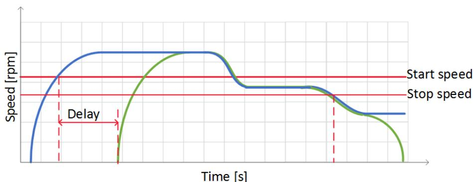
*Fig. 1.7 Staging up the number of working pumps. Working application is ABB Pump Control software based on ACQ810 frequency converter. The graph is stored by ABB DriveStudio VSD monitoring tool.*
