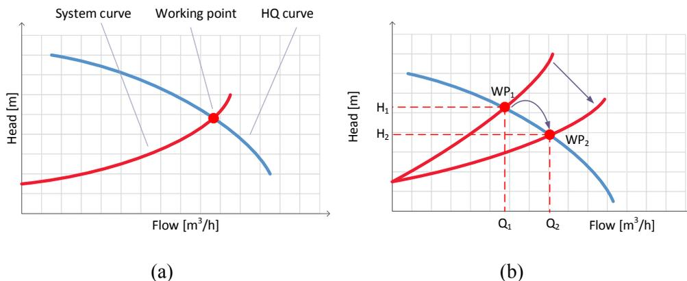
Fig. 1.3 Location of the working point in the steady state (a) and in the case when the conductivity of a pipeline increases.
