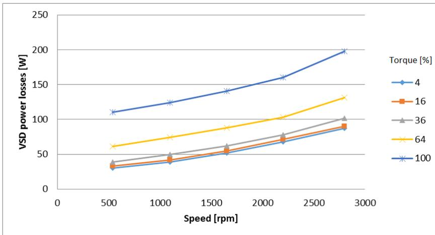
Fig. 3.11 Characteristics of the VSD, representing the dependence between pump speed and drive losses. The graph shows power losses of ABB ACQ810-04-06AD-5,  $P_{nom} = 1.1 \text{ kW}$  and M3BP90LB2 2 pole asynchronous motor with  $P_r = 1.5 \text{ kW}$  and  $n_r = 2892 \text{ rpm}$ .
