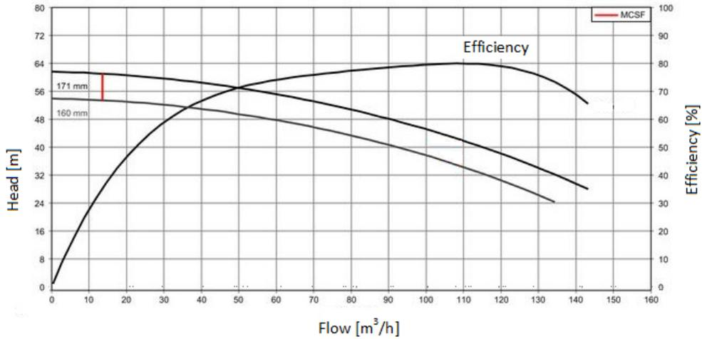
Fig. 1.15 Characteristic curves of Ebara 3UB-65-200 centrifugal pump for impellers of diameter 171 mm and 160 mm .
