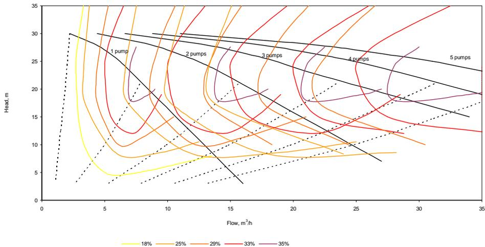
*Fig. 3.3 Efficiency distribution across the performance and system characteristics of five parallel-connected pumps Ebara CDX 120/12.*
