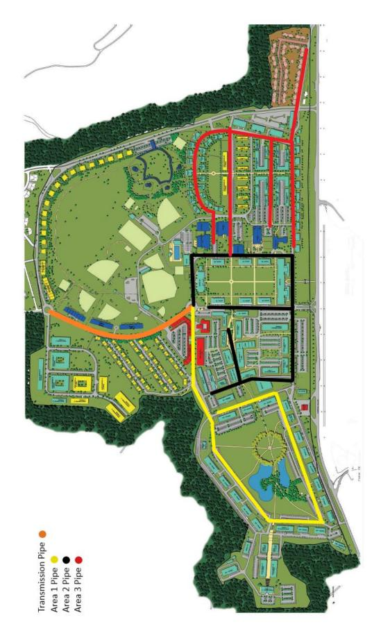
Figure 2.6 Map depiction of the pipeline network as implemented by subarea. Map from [44]
