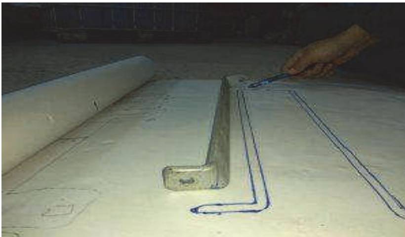
Picture 3: Imprinting of some complicated parts from the DIY legume-harvesting machine made by Nikos Stefanakis and the Melitakes group
