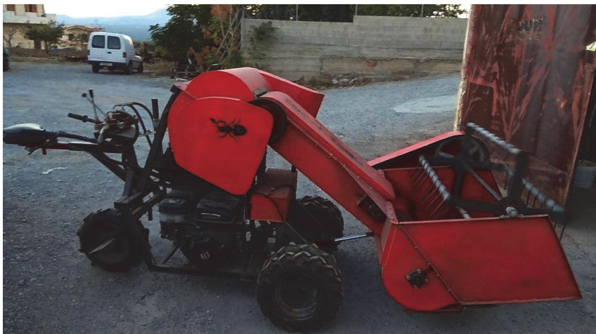
Picture 1: DIY legumes harvesting machine by Nikos Stefanakis and the Melitakes group
