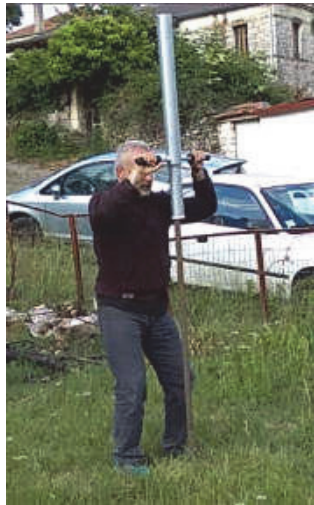
Picture 4: Testing the newly constructed tool for hammering fencing-poles from the Tzoumakers group
