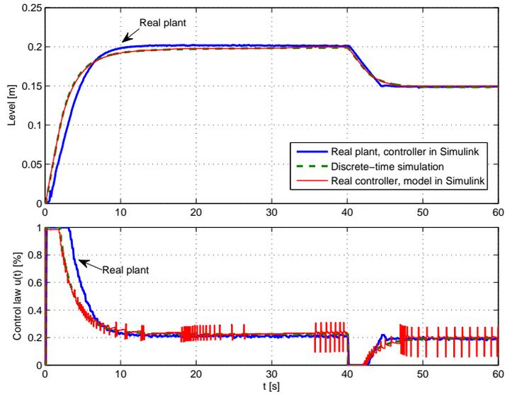
Figure 7.4: Level control with set point change
