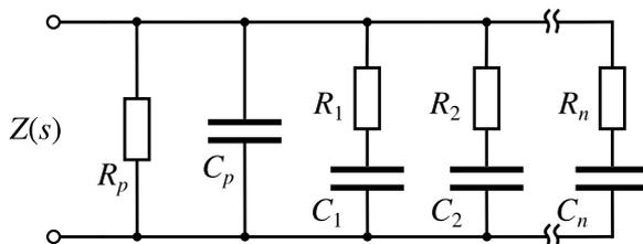
Figure 5.7: Foster II form canonical RC network
