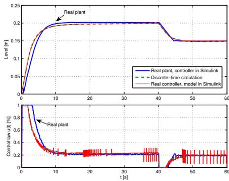
Fig. 6. Level control with set point change
