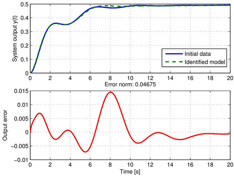
Figure 6.4: Indirect method: time domain validation
