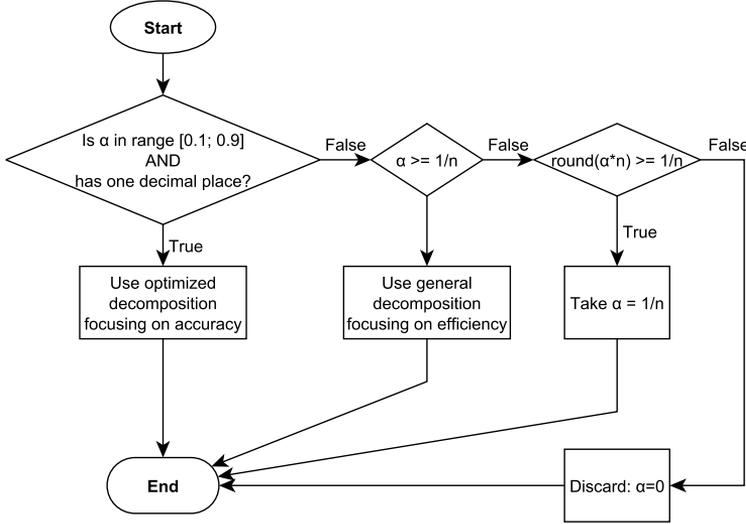
Figure 5.2: Order  $\alpha$  decomposition algorithm
