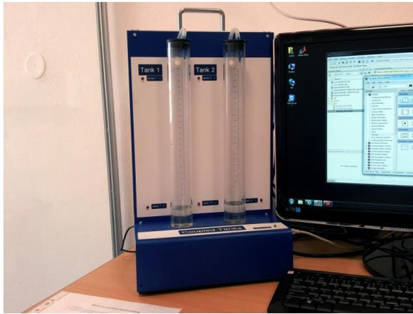
Figure 7.2: The coupled tanks system laboratory plant
