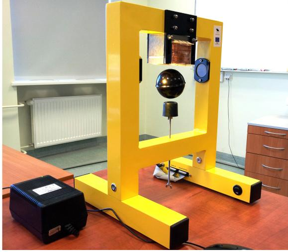
Figure 7.11: Real-life laboratory model of the MLS
