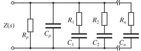
Fig. 2. Foster II form canonical RC network
