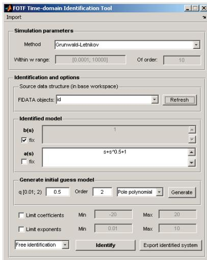
Fig. 8. FOTF Time-domain Identification Tool user interface
