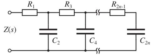
Fig. 1. Cauer I form canonical RC network
