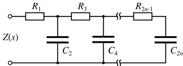
Figure 5.6: Cauer I form canonical RC network
