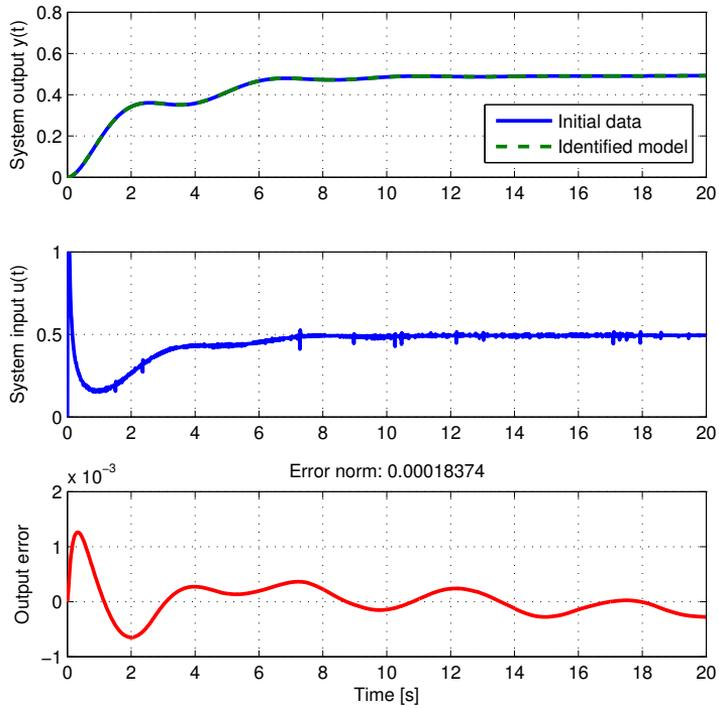
Figure 6.6: Direct method: time domain validation
