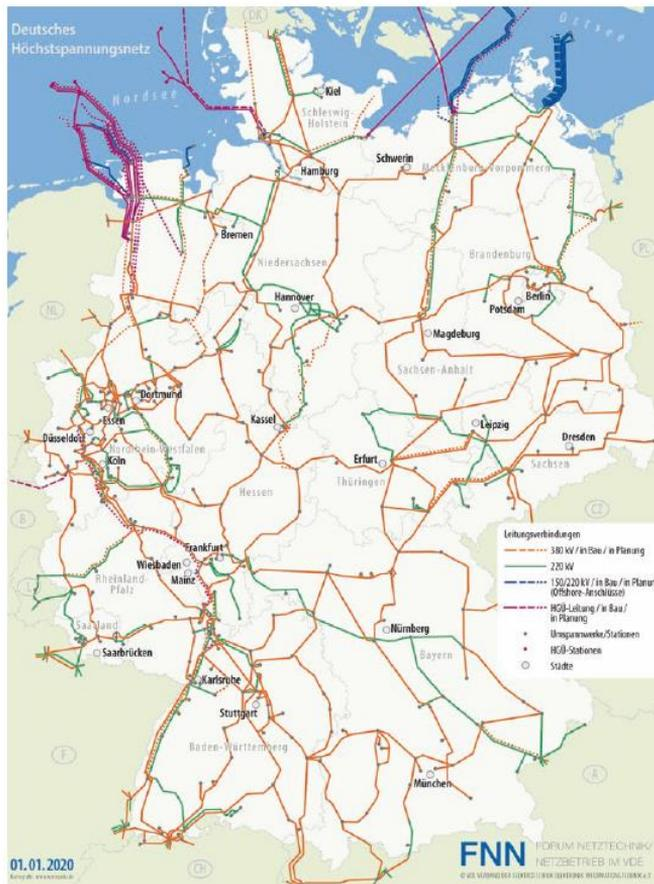
Figure 2-10. German 380 kV and 220 kV EHV level including HVDC networks (Schäfer K. , 2022).
