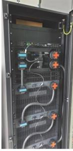
Fig. 2. Home battery energy storage system I (HBESS<sub>1</sub>).
