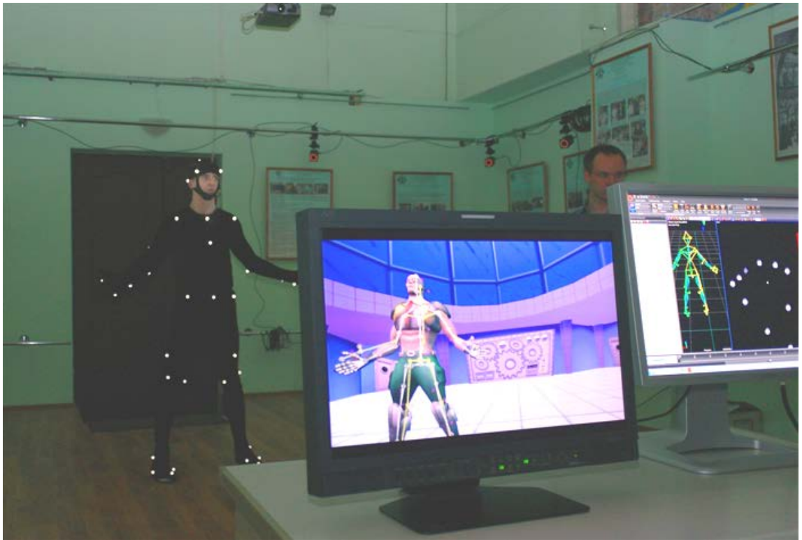
Figure 7 Shooting area. Actor in costume, his skeleton in Blade (right) and 3D model based on Skeleton (left)
