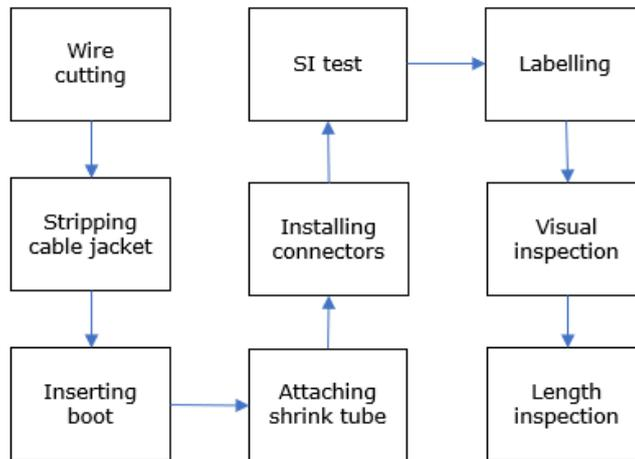
Figure 2.1 (Sample) production and testing process (Jem Electronics, 2018)
