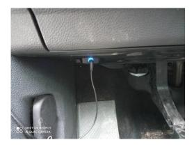
Figure 9. GoFar OBD-II dongle connected to Volkswagen Golf's OBD-II port
