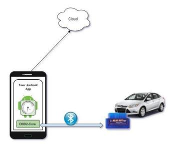
Figure 10. Sample OBD-II device communication diagram [32]
