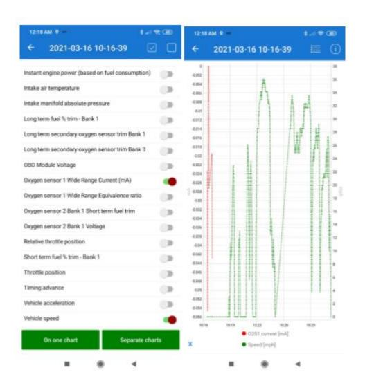
Figure 15. Oxygen sensor 1 and vehicle speed data from Veepeak OBDCheck
