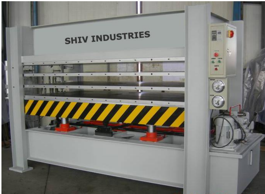
Figure 1.7 Hot pressing of Particleboard
