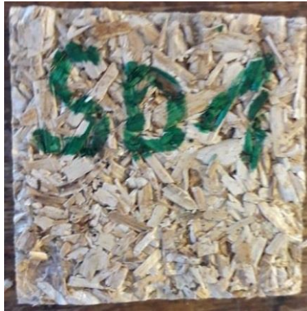
Figure 2.5: Thickness Swelling test sample
