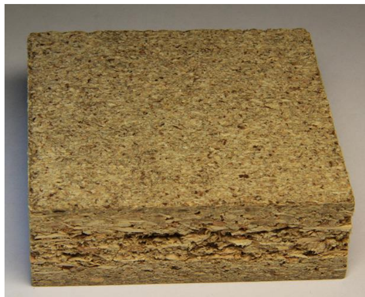
Figure 1.1 Three – layered particleboard (Wang, D., Sun, X.S., 2002)
