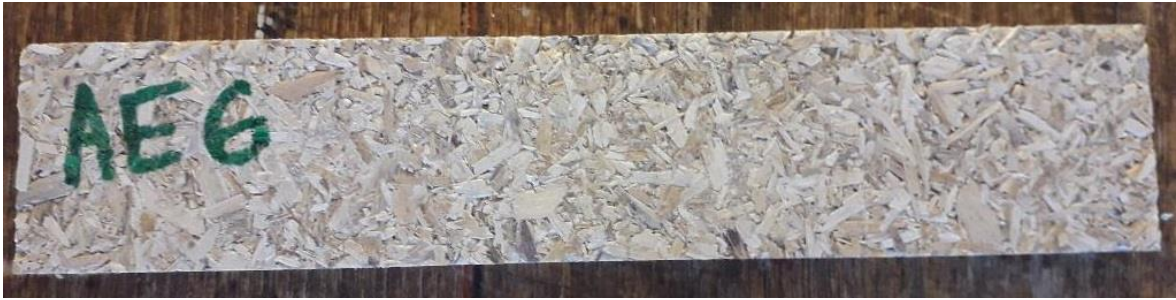
Figure 2.3: Flexural Strength test sample
