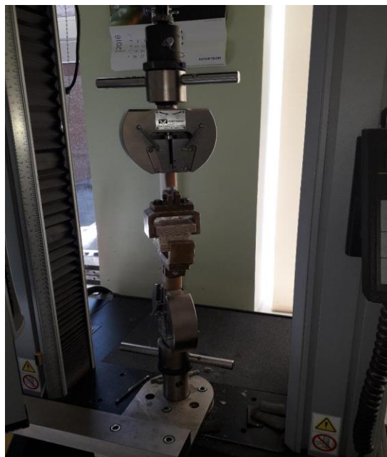
Figure 2.2 Tensile strength perpendicular to the plane of the board
