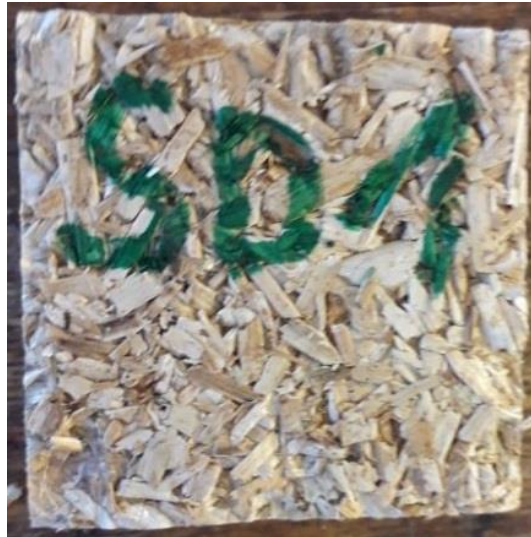
Figure 2.1: Tensile Strength test sample
