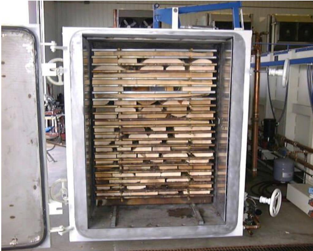
Figure 1.3 Kiln Drying (Sam-Brew S., 2017)
