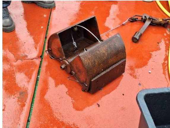
Figure 13. Grab sampler used for surface sediment and Fe–Mn concretion sampling (personal archive).
