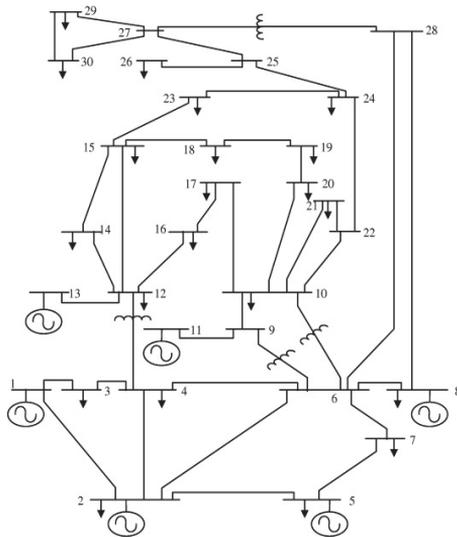
Figure 3.7. IEEE 30-bus test system[69]
