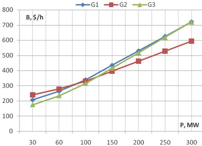
Figure 3.10. Model II. Fuel-cost characteristics of generators
