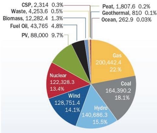
Figure 1.3. EU power mix in 2014 in MW[2]
