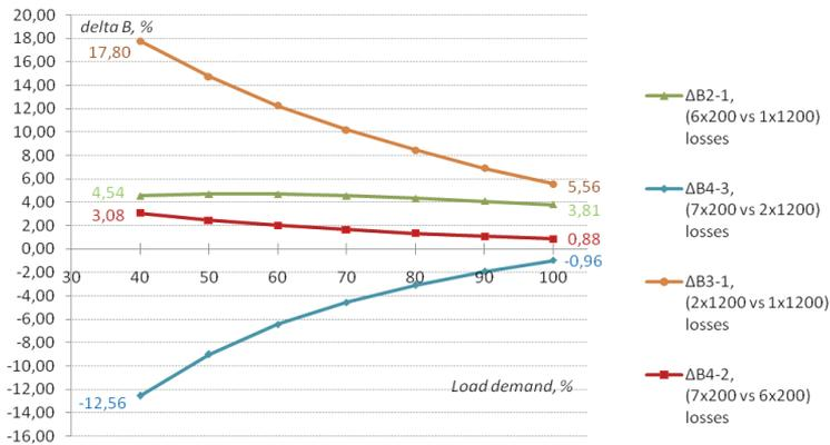
Figure 3.5. Difference in fuel consumption considering power losses. Model I. Fuel: coal
