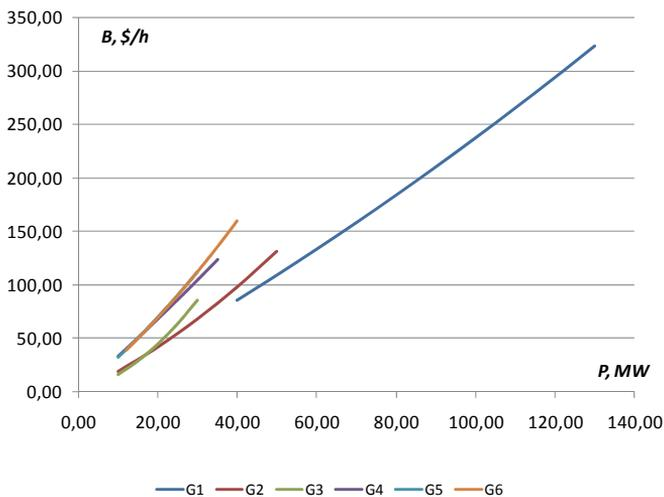
Figure 3.16. Fuel costs characteristics of generation units
