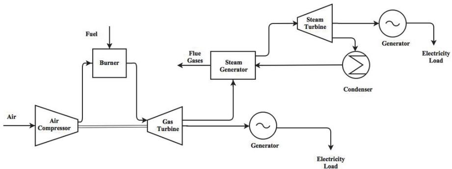
Figure 2.1. Typical scheme of thermal condensing power plant [4]
