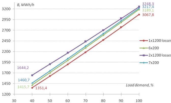
Figure 3.4. Fuel consumption considering power losses. Model I. Fuel: coal.
