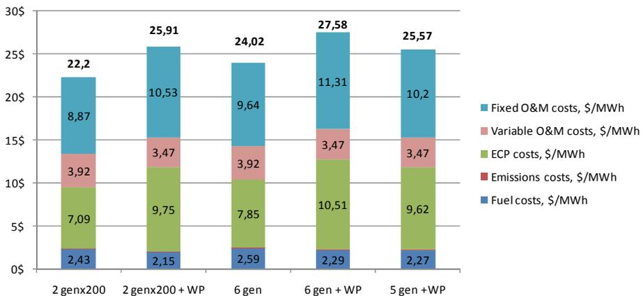
Figure 3.19. The final comparison of models
