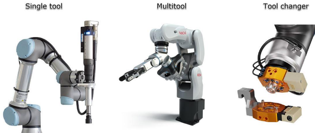
Figure 1.4.1. Options for attaching the EOAT to the robot arm [25], [26], [27]
