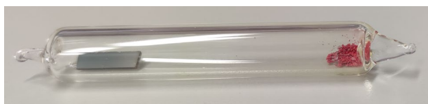
Figure 8. Sb_2Se_3 thin film and SbI_3 powder inside a sealed quartz ampoule.
