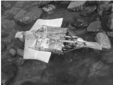
Fig. 45. The third prototype with redesigned fins and an additional joint.
