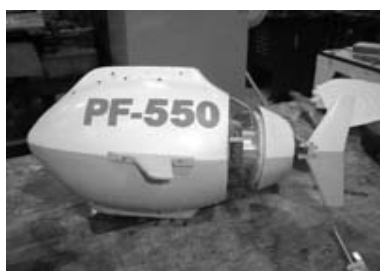
Fig. 18. Experimental model of PF-550, built for study up-down motion mechanism
