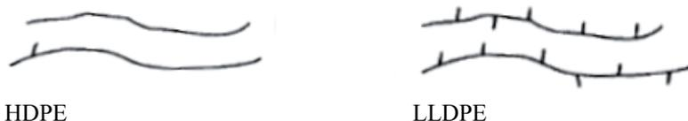
Figure 7. Different polyethylenes
