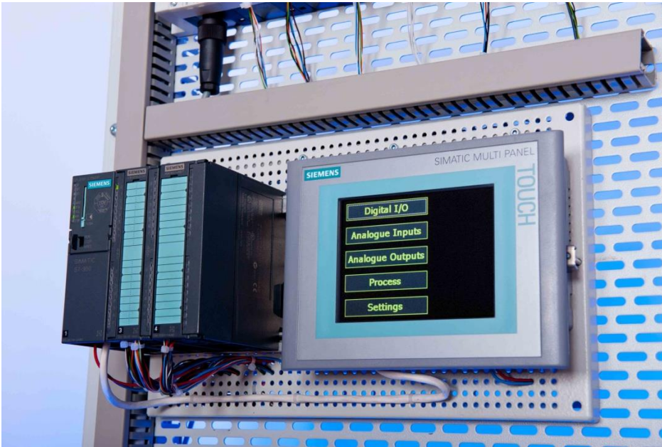
Figure 5.11 Siemens S7-300 controller and control block
