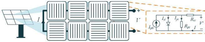
Figure 3.2 PV module layout and equivalent circuit model of solar cells connected in the series format.
