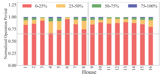
Fig. 5. Share of each operation power for the main isolated bidirectional ac-dc converter in the buildings. (colors show the operating power level).
