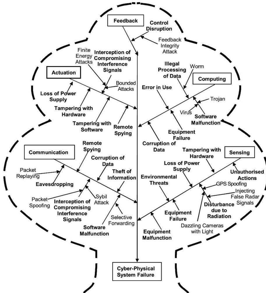
Figure 8: Tree diagram of attacks and threats on CPS (Source [36])
