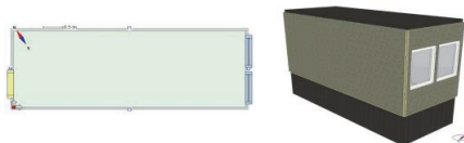
Fig. 3. The container model in IDA ICE with floorplan on the left and 3D view on the right. The compass is shown for orientation in both pictures
