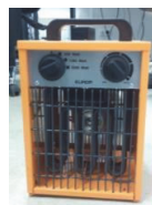
Fig. 2. EUROM electric heater placed in the middle of the control center for calibration measurement
