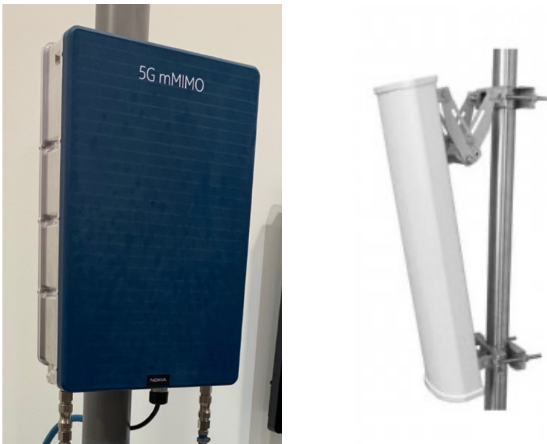
Figure 1.2 Comparison of AAS manufactured by Nokia (on the left) [7] and passive antenna manufactured by Varius (on the right) [8].
