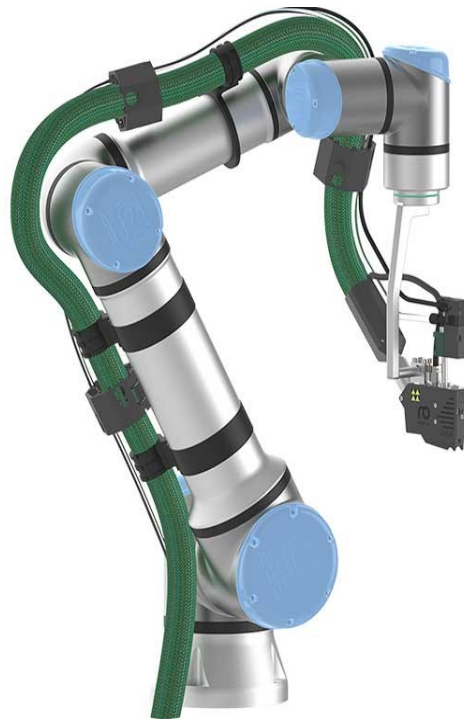
Figure 4.2.1 UR10 with hose and EOAT for glue dispensing [41]
