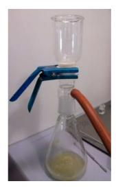
Figure 12. Filtration under vacuum setup.
