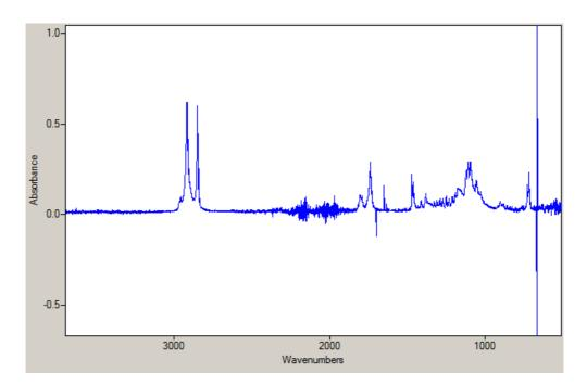
Figure 33. Cellulose stearate spectrum. Synthesis 1:5 with catalyst.
