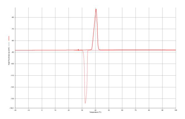
Figure 26. Calorimetry graph of cellulose stearate obtained from synthesis 1:5 without catalyst and carried out with high purity stearoyl chloride.
