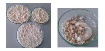
Figure 18. CS obtained. (Left image) Up on the left: synthesis 1:5 with catalyst, up on the right: synthesis 1:3 with catalyst and down: synthesis 1:5 without catalyst. (Right image) synthesis 1:1.
