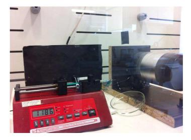
Figure 39. Electrospinning setup.
