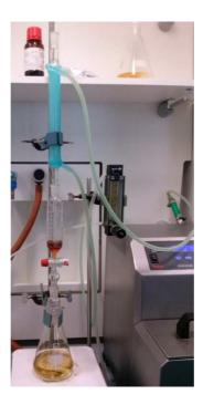
Figure 10. Setup for Cellulose Stearate obtention.
