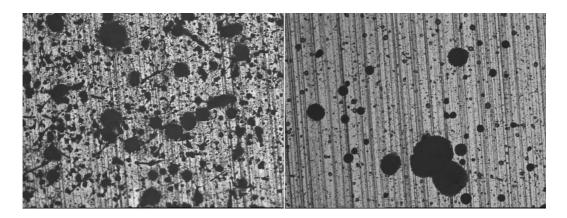
Figure 40. Microscope images. On the left *4 chloroform : 1 DMSO and 10* and on the right 8 *chloroform : 1 DMSO and 10%*.
