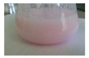
Mixture after titration with NaOH.
