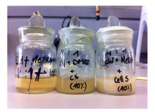
Figure 38. Examples of electrospinning mixtures. The one on the left is suitable for electrospinnig, the one in the middle is too viscous and the on the right, the polymer is precipitated.
