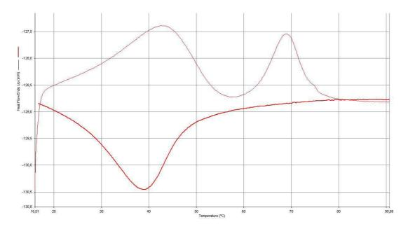
Figure 22. Calorimetry graph of cellulose stearate obtained from synthesis 1:3 with catalyst.
