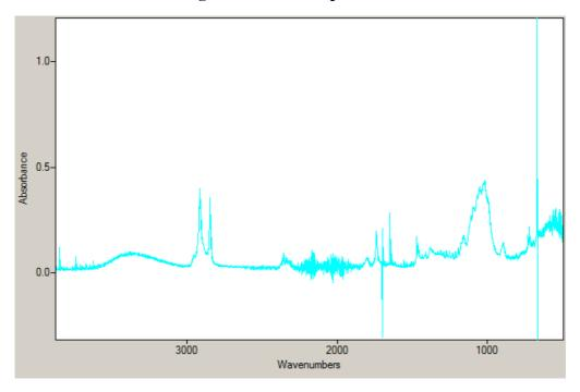
Figure 35. Cellulose stearate spectrum. Synthesis 1:1.
