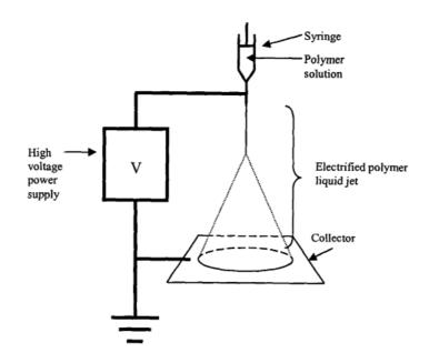
Figure 8. Schematic diagram of the electrospinning process. [44]
