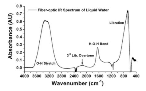
Figure 28. IR spectrum of liquid water [55]
