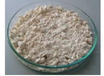
Synthesis 1:5. Polymer obtained after drying it in the oven.
