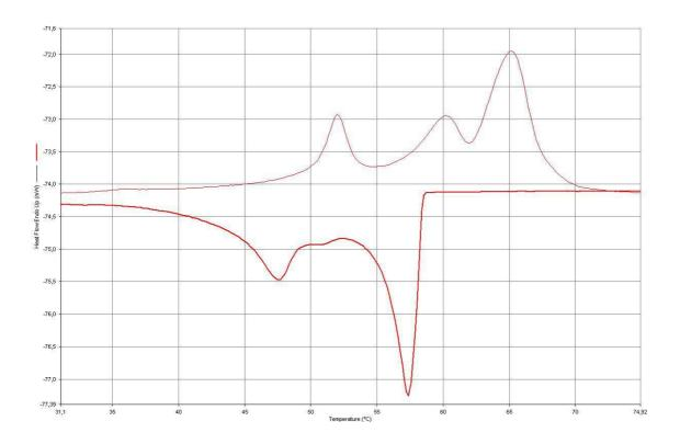
Figure 20. Calorimetry graph of cellulose stearate with 0,46 DS ( synthesis 1:1 without catalyst).
