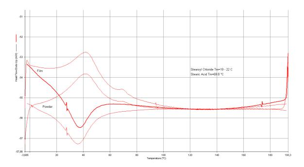
Figure 21. Calorimetry graph of cellulose stearate with 0,53 DS (synthesis 1:3 without catalyst).
