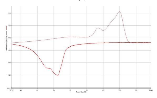
Figure 24. Calorimetry graph of cellulose stearate with 0,78 (synthesis 1:5 with catalyst).
