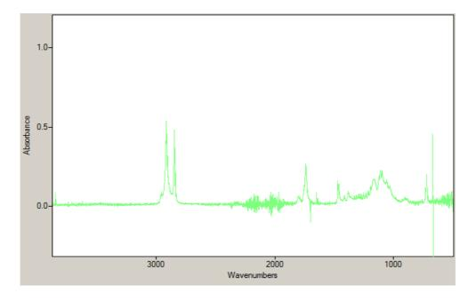
Figure 32. Cellulose stearate spectrum. Synthesis 1:5.
