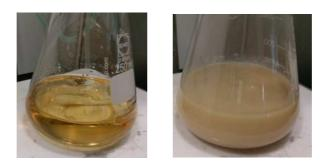
Figure 11. On the left: mixture of IL, cellulose and stearoyl chloride. Start point of the reaction. On the right: polymer obtained after 3 hours of reaction.
