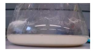
Polymer mixed with methanol. Two phases can be observed.
