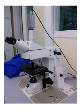
Microscope used for evaluation of electrospinning results.
