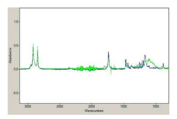
Figure 37. FTIR spectra of 1:5 synthesis done with all compounds of technical purity (green line) and technical purity IL but high purity stearoyl chloride (blue line).
