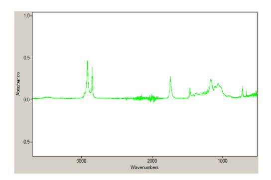
Figure 31. Cellulose stearate spectrum. Synthesis 1:3 with catalyst.
