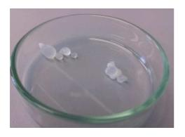
Cellulose that has not been dissolved correctly in the IL.
