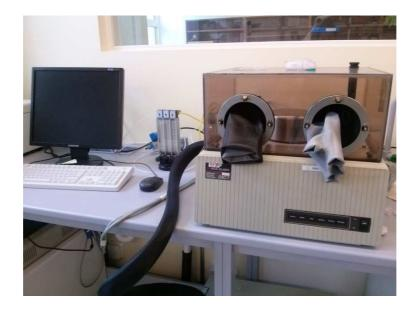
Differential Scanning Calorimeter.
