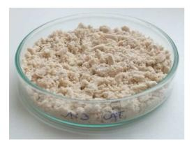
Synthesis 1:3 with catalyst. Polymer obtained after drying it in the oven.
