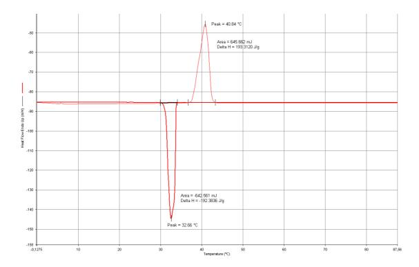
Figure 25. Calorimetry graph of cellulose stearate obtained from synthesis 1:5 without catalyst and carried out with high purity reagents.
