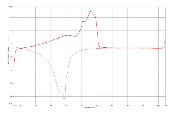
Figure 23. Calorimetry graph of cellulose stearate with 0,55 DS (synthesis 1:5 without catalyst).
