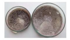
Figure 19. Polymers obtained by using high purity stearoyls chloride and technical purity IL (on the left) or high purity IL (on the right).
