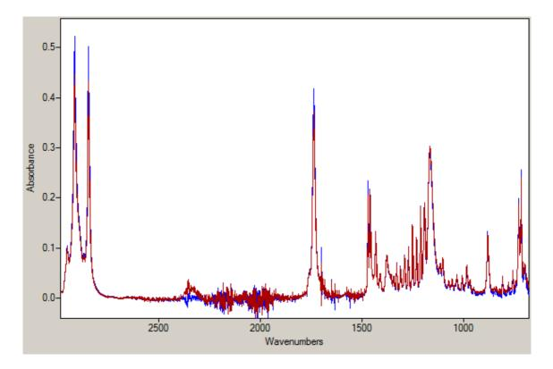
Figure 36. FTIR spectra of 1:5 synthesis done with high purity IL (blue line) and technical purity IL (red). In both cases high purity stearoyl chloride is used.
