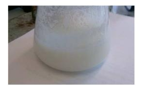
Mixture after titration with HCl.
