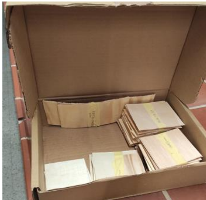
Figure 1 The prepared specimens of birch, aspen, black alder and gray alder
