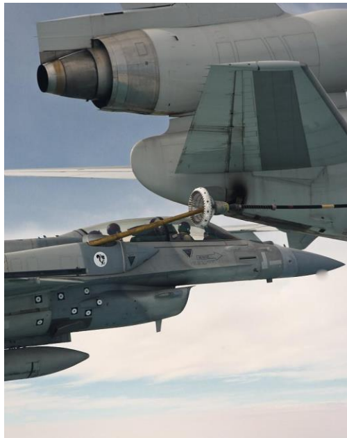
Figure 1.5 Probe-and-drogue system in aerial refueling [4]
