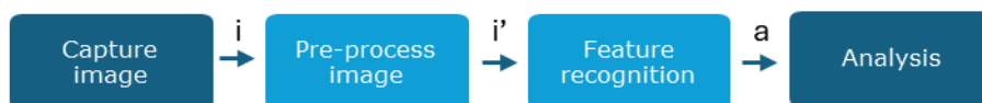
Figure 2.2 Image processing pipeline, where i is the captured image, i' is the pre-processed image and a are the abstract features.
